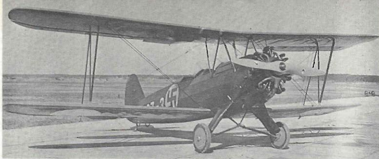
Right: Focke-Wulf Stieglitz trainer (SZ-3) soon after delivery from Germany in the late thirties. (E. Ritaranta via C. F. Shores).
