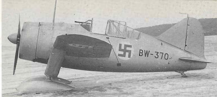
Left: Brewster 239 fitted experimentally with skis during the period between the wars. Note this aircraft is painted in U.S. Navy pale grey. (E. Ritaranta).
