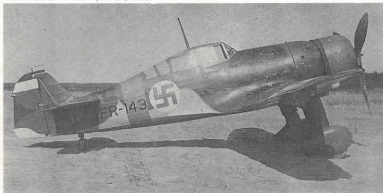
Above: The first V.L.-built Fokker D.XXI with Pratt and Whitney Twin Wasp Jr. engine and all-wing mounted armament. This aircraft has been finished in the black and green camouflage scheme, but carries no yellow identification markings, indicating that this photograph was taken before the start of the Continuation War. The aircraft is FR-150. (G. Kamphuis).
