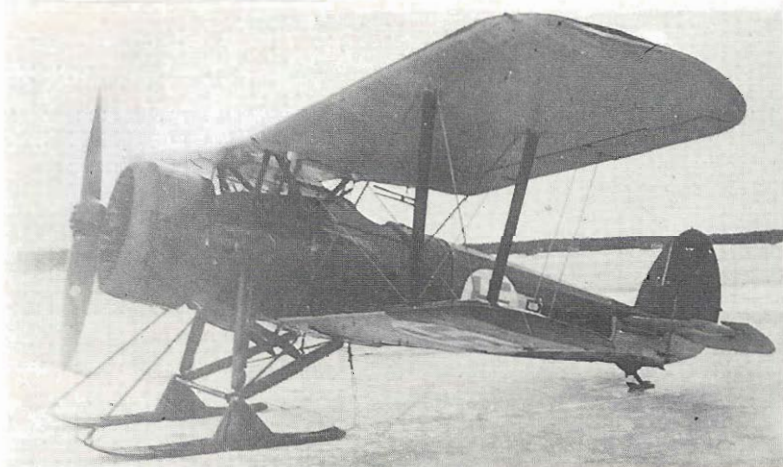
Below: Also used for fighter training after replacement by Gloster Gladiators in HLeLv 26, was this ski-equipped Bristol Bulldog IVA. (E. Ritaranta via C. F. Shores).
