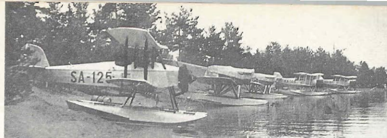
Line of floatplanes on the edge of a typical Finnish lake. The nearest aircraft is a V.L.Saaski II (SA-125), then come two A-22s, and further away are a pair of V.L.Kotka IIs (KA-146 and 148) (E. Ritaranta).
