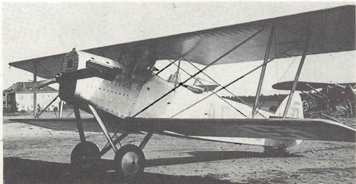
Aero A-32 reconnaissance-bomber of the Detached Ground Flight Squadron at Suur-Merijoki. The aircraft is coded AEI-45. Note fighter Koolhoven FK-31 (KO-35) in the background. (E. Ritaranta).
