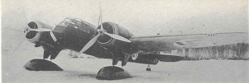
Above: One of the first Bristol Blenheim Is to be delivered from England, BL-104 is here seen fitted with skis shortly after arrival. (J. Alexander via C. F. Shores).
