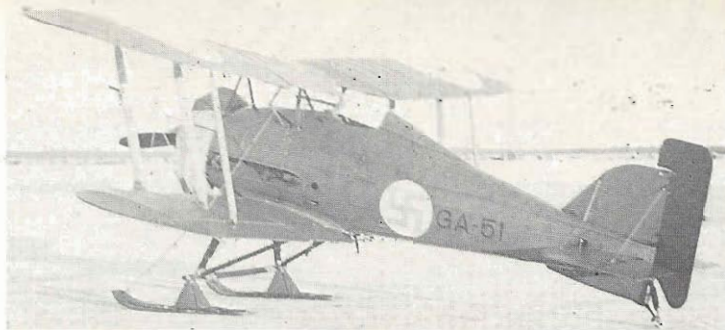
Left: Gloster Gamecock II used during the Winter War for fighter training after being replaced in HLeLv 24 by Fokker D.XXIs. GA-51 is seen here fitted with skis for winter operations at Kauhava. (E. Ritaranta).
