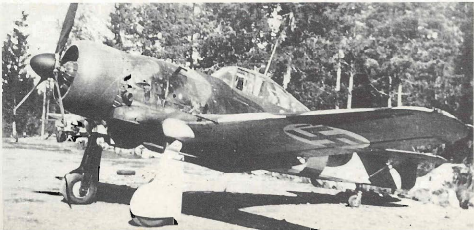
Below: D.XXI (Twin Wasp Jr.) FR-107, experimentally fitted with a retractable undercarriage. The small improvement in performance did not warrant production of the type. (G. Kamphuis).
