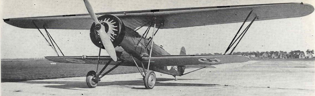
Above: Fokker C.V.E. (FO-65) in factory-fresh paintwork, immediately after delivery. Note that this aircraft still retains the Townsend ring cowling at this stage. (G. Kamphuis).
