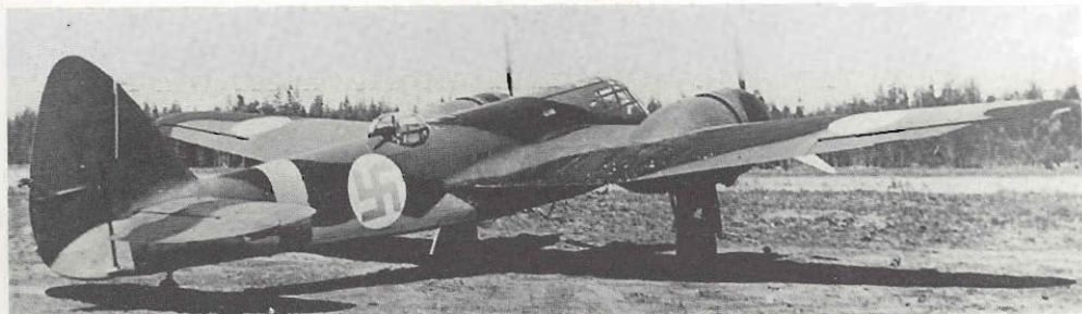
Above: Blenheim I BL-115. This aircraft is carrying a German 7.7mm. MG 34 machine gun in the dorsal turret in place of the normal Lewis gun. (E. Ritaranta via C. F. Shores).
