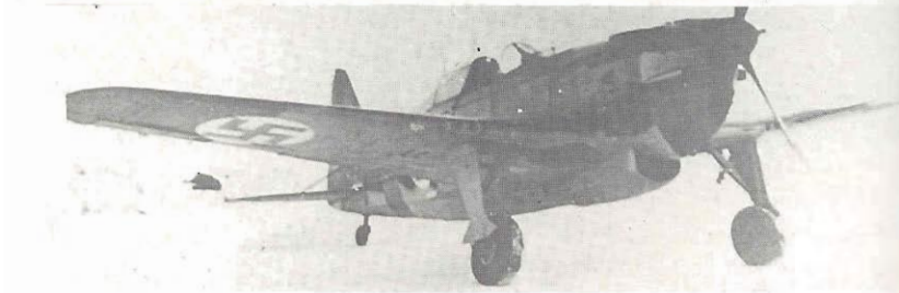
Above: A Morane 410 with four (wing-mounted) machine-guns instead of the usual two. This aircraft was one of the final batch of Moranes supplied to Finland in 1943. (G. Botquin via C-J. Ehrengardt).
