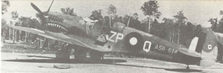
Above: Spitfire Mk. VIII A58-614 in dispersal area at Morotai. Note the high join of upper and under surface camouflage. No. 457 Squadron, No. 80 Fighter Wing, No. 1 Tactical Air Force, Royal Australian Air Force.
