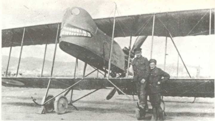
Above: Maurice Farman Fighting Bus, No. 2 Wing, Royal Naval Air Service, Imbros, Aegean Sea late 1916 early 1917. As the Lewis gun was raised or lowered the mouth opened and closed. One of the first examples of a Sharkmouth on a British aircraft. (via J. M. Bruce)
