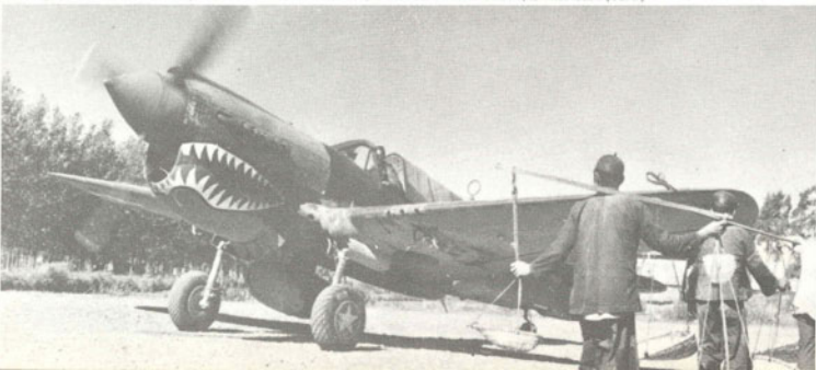
Below: Nice shot of a P-40N Warhawk of the 23rd Fighter Group taxiing past a convoy of Chinese earth movers. Apparently an OD and grey aircraft with sand cowf panels cannibalised from another a/c. Blue and red mouth, blue lips, white teeth. (USAF)
