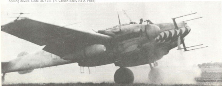
Below: An ex ZG76 Bf 110G night-fighter of Stab. 1/NJG4, note long-range tanks and wing-tip aerials for the Flensburg radar homing device. Code 3C+LB. (R. Carson Seely via A. Price)
