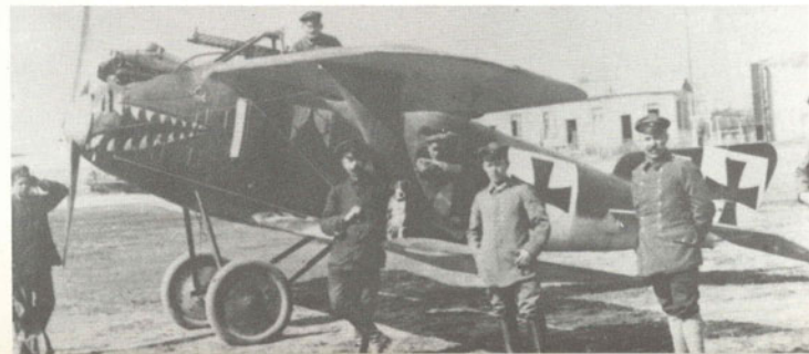
Below: One of the earliest known examples of a Sharkmouth, see colour illustration. Note Spandau machine gun mounted on nose, modified crash pylon and painted curtains on side windows. (via Peter M. Grosz)
