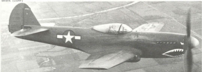
Above: The one and only XP-40Q here shown with clipped wings, see colour illustration. (via Peter M. Bowers)
