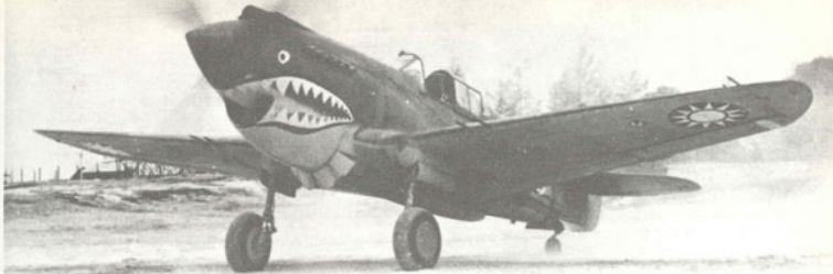
Above: Nice shot of an AVG Tomahawk IIB about to take off from an airfield near Rangoon, Burma. Number in white on fuselage of this aircraft is believed to be 5, see colour illustration. Other numbers known to have been carried by Tomahawks during the defence of Rangoon are: 9, 55, 56, 71 and 74 all with thin red fuselage band. Note the underwing roundels are slightly further outboard than the upper surface ones. (IWM)
