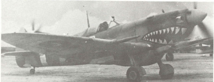
Above & below: A pair of Mk VIII's of No. 457 Squadron on Morotai airfield. Standard RAF scheme of grey/green uppers, pale grey unders. Aircraft above is ZP-B, A-58-611.
