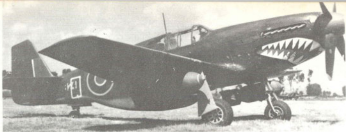
Above: GA-Q FB241, a North American Mustang Mk. III of No. 112 'Shark' Squadron on an Italian airfield. Standard green/grey upper surfaces with pale grey under surfaces, Black/red mouth, white teeth, black lips.
