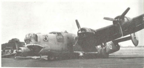
Right: This B-24J of the 93rd Bomb Group, 330th Bomb Squadron, 8th Air Force, flown by Lt. Ches Agee ran out of runway through lack of brakes due to flak damage over Germany. The mouth in actual fact was supposed to represent a Whalemouth and not a shark. Code AG+L, serial unknown. (Ches Agee via Stan Staples)
