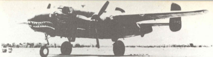
Above: Sharkmouthed B-25C Mitchell, the 10th aircraft modified with solid nose. 'Mortimer' on nose in white, row of five Jap flags under cockpit, serial 112443, Unit unknown.
