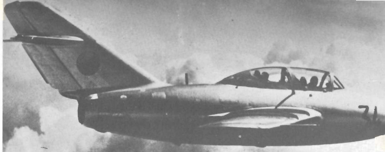
Above: CS-102 (MiG-15UTI) two-seat fighter-trainer, the black 34 on the nose is a factory and not a service designation.
