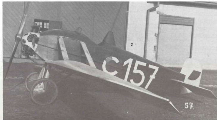
Below: Avia BH-10 designed and built for aerobatic training, first flown in 1924 with Walter NZ 60h.p. engine. Central Flying School, Prostějov, Moravia.
