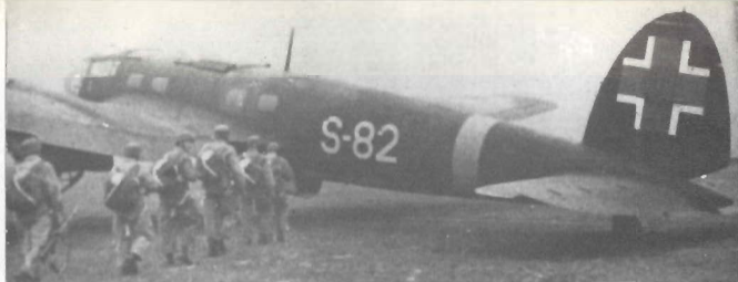
Above: Heinkel He 111H, Slovak A.F. Note the blue cross with red disc tail marking, yellow fuselage band (and wing tips) and white code, standard Luftwaffe splinter scheme.
