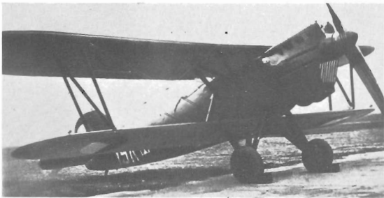
Aero A-100 bomber, 1st Air Regiment, Prague, 1933. Powered by a 650h.p. Avia Vr-16 engine.
