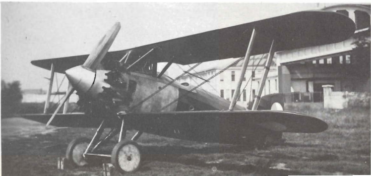
Below: Letov S-31 powered with a 480h.p. Walter Jupiter engine, thirty-two were delivered during 1932.
