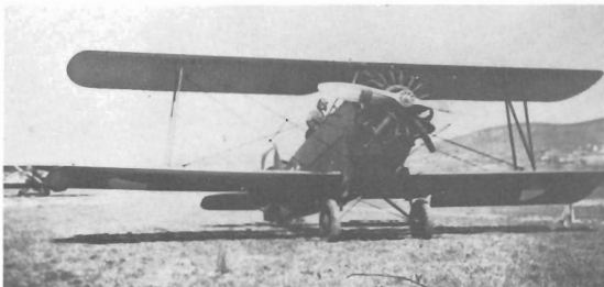
Avia BH-26 two-seat fighter of 1927 powered by a Walter Jupiter IV of 450h.p., 3rd Air Regiment, Nitra airfield, Slovakia.
