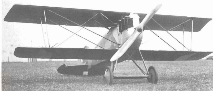
Below: Aero A-18 fighter biplane with BMW IIIa 185h.p. engine, 1st Air Regiment, Kbely airfield, Prague 1923. Twenty A-18's were delivered to the Cz.A.F.
