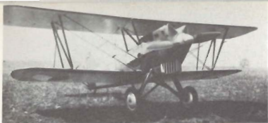
Above: Avia B-534 of early production batch, note radiator under cowl and open cockpit.
