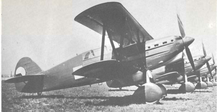
Line-up of Avia B-534 biplane fighters of the fourth production series with enclosed cockpit prior to delivery to squadrons.
