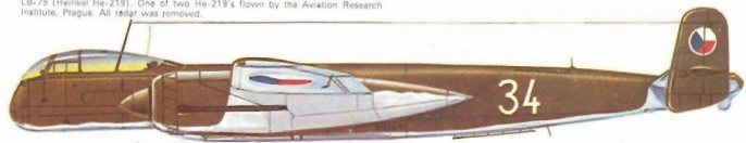
6 LB-79 (Heinkel He-219). One of two He-219's flown by the Aviation Research Institute, Prague. All radar was removed.
