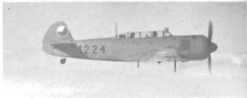
Above: C-11 (Yak-11) advanced trainer with ASh-21 700h.p. engine built under licence by SPP Kunovice.
