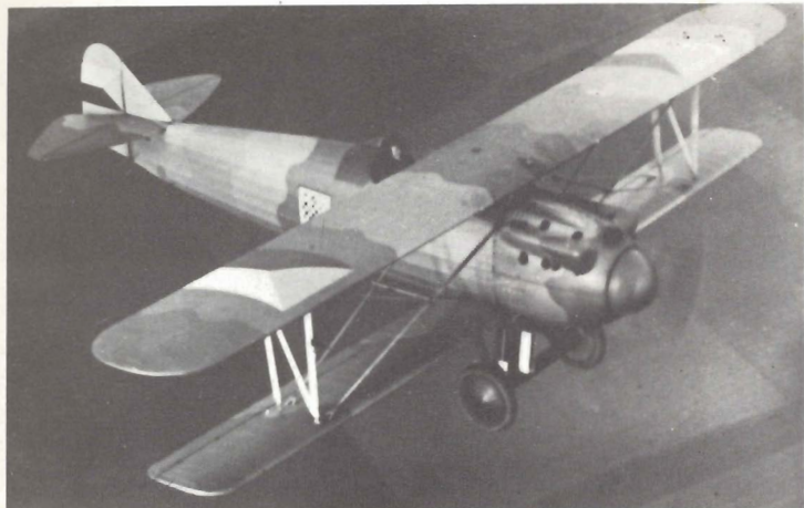
Above: Letov S-20 fighter powered with a Skoda HS 8Fb engine of 300h.p., of the 2nd Air Regiment, Olomouc. 95 were delivered to the Cz.A.F. and a small series to the Lithuanian A.F.
