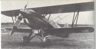
Above: Avia B-534 of the third production series with Avia HS 12Ydrs engine of 850hp.
