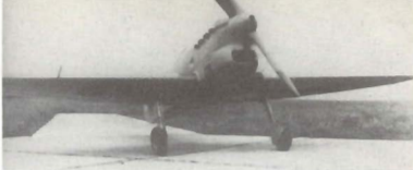
Above: Avia B-135 prototype with retractable u/c, twelve were delivered to the Bulgarian A.F. in 1941.
