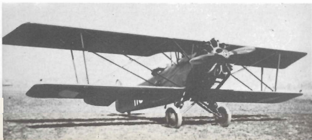
Below: Aero A-32 of the 3rd Air Regiment on Priestany airfield, 450 h.p. Walter Jupiter. Sixteen A-32's were delivered to the Finnish A.F., in 1929.
