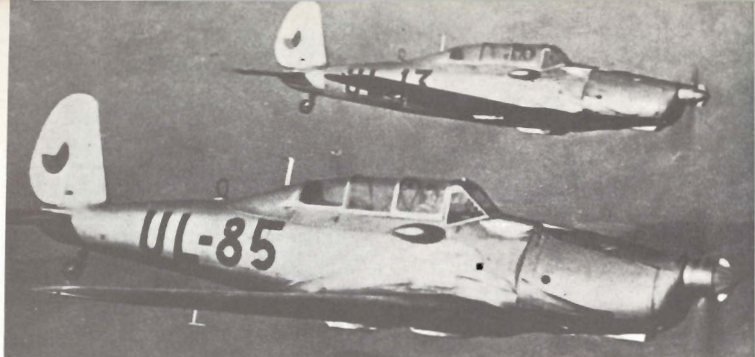
Above: C-2 (Arado Ar.96B) trainer. Note camera-gun pod beneath front cockpit. 394 C-2's were built by Avia and Letov factories during 1945-49.
