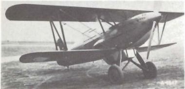
Above: Avia Bk-534, a cannon-armed version with the HS Ycvs 850hp engine.
