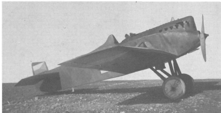
Above: Avia BH-3 fighter of 1921 powered by a Walter W-IV engine of 220h.p. Ten aircraft only of this type were delivered.
