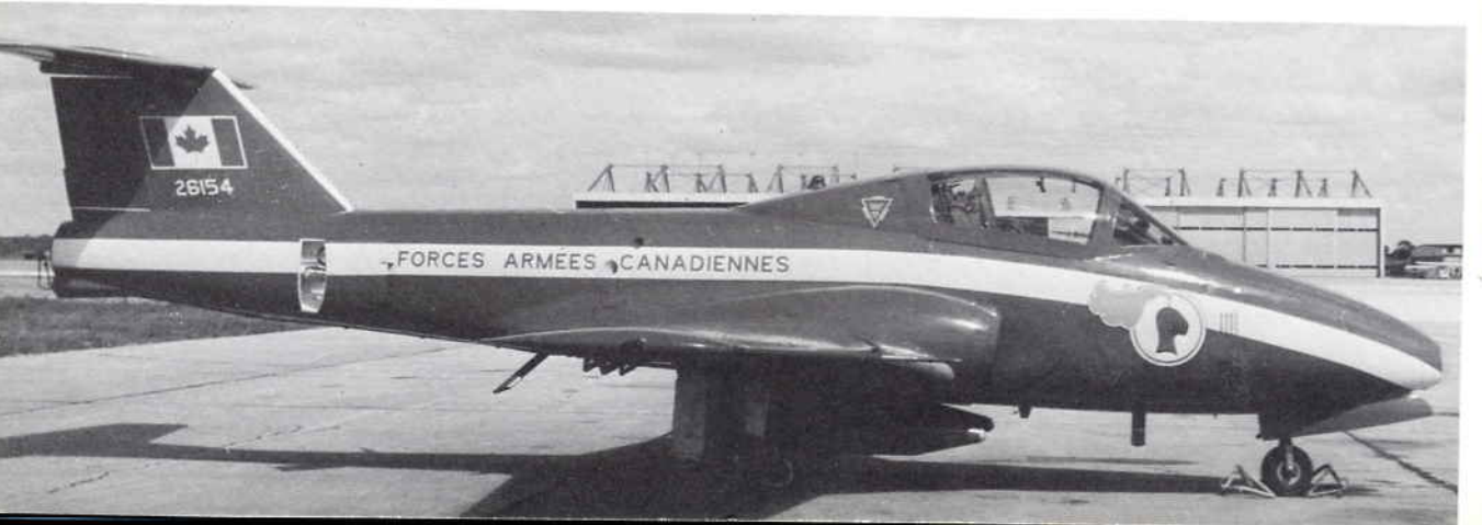
Below: A spick and span Canadair CL-41A Tutor of the RED KNIGHTS, Canadian Armed Forces, note smoke making apparatus under the fuselage. (S. P. Peltz)
