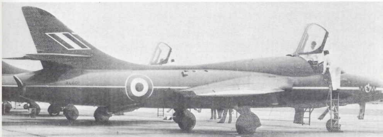
Below: Another T.7 of the BLUE DIAMONDS showing starboard side details, aircraft letter T in black above fin flash, serial XL605 in black above white cheat line. (S. P. Peltz)
