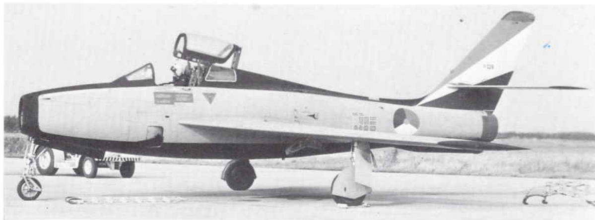
Above: Republic F-84F Thunderstreak of WHISKEY FOUR of the Royal Netherlands Air Force, serial is P-228. (S. P. Peltz)
