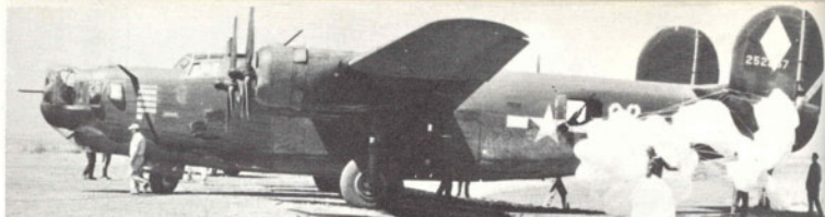
Above: Olive drab B-24J of the 456th Bomb Group with a rudder from a 485th BG aircraft, see side-view illustration E2. Below: Another B-24J of the 455th BG in natural metal finish, see side-view illustration E2. Both aircraft had their hydraulics damaged in combat and resorted to parachutes fastened to the beam gun mounts to shorten the landing roll. (USAF)
