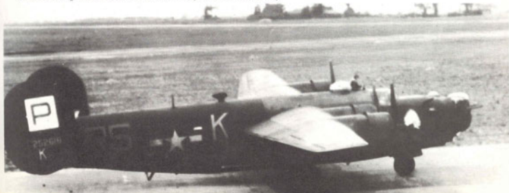
• Below: B-24H "Chief Wapella" of the 487th Bomb Group, 839th Bomb Squadron. Note square presentation of Group letter repeated on upper surface of starboard wing. See colour side-view illustration F6. (USAF via R. J. Francillon)
