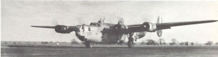
Below: A crew chief signals stop engines as this B-24J of the 458th Bomb Group, 755th Bomb Squadron arrives on its dispersal area. The nose of this aircraft appears to have been painted yellow in the same style as some aircraft of the 93rd BG painted theirs red. (USAF via R. J. Francillon)
