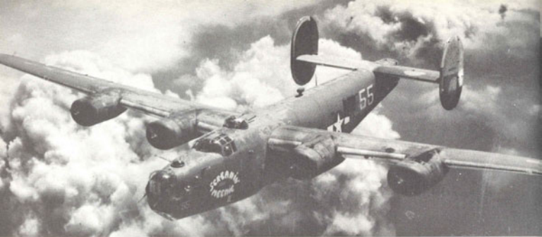
Above: "Screamin' Meemie II" a B-24J of the 451st Bomb Group in full Group tail markings, OD and grey scheme without de-icer boots. Photo was taken during the 15 July 1944 raid on Ploesti, Rumania. (USAF)
