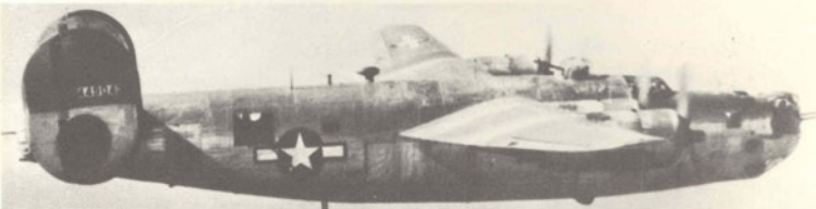
Above: A B-24M of the 451st Bomb Group, 728th Squadron, standard group colours on tail, serial 449043, red 5 on dirty square on aft fuselage, note RCM aerial. (USAF via R. J. Francillon)
