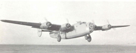
✓ A B-24D of the 376th Bomb Group, 9th Air Force coming in to land at Solluch LG, near Benghazi, Libya after the first Floesti raid. Desert sand and pale blue scheme with white 88 on nose and fin, RAF fin flashes and early insignia without surround and white bars. De-icer boots on all leading edges. (USAF)
