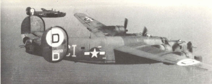
• Above: Olive Drab and grey B-24H of the 392nd Bomb Group, 576th Bomb Squadron heading out over the English Channel for a target somewhere in Europe. Note the white disc on tail and upper wing surfaces, aircraft letter D and serial 129433 in yellow, code CI in pale grey. Note near straight demarcation line between OD and grey. (USAF via R. J. Francillon)
