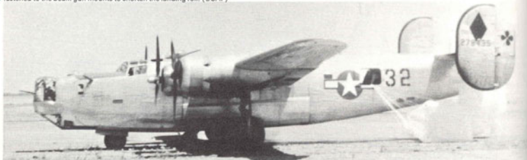
Left: B-24J of the 454th Bomb Group after running out of runway on landing, probably due to damage during combat to the hydraulic system. Note the extended black area on the tailplane, black 7 on fuselage and de-icer boots fitted.
