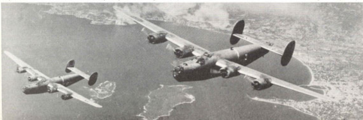
A pair of B-24H's of the 450th Bomb Group complete with Wing/Group symbols on tailplane and vertical surfaces. Note white fuselage band. (USAF)
