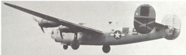
Below: A B-24H of the 304th Bomb Wing, without definite knowledge of the colour of the lower half of the fin the group cannot be determined, the colour is either white or yellow, 454th or 455th Bomb Group, the 455th seems to be the more probable, serial is 128914. Note 506 on nose and de-icer boots on vertical tail surfaces. Attack was on La Spezia on 22 May 1944. (IWM)
