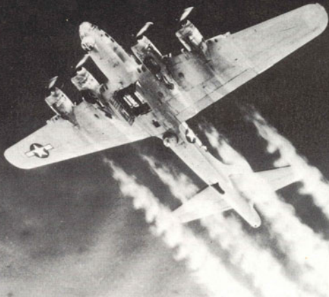
B-17G, probably of the 355th BG on its bomb-run, OD and grey scheme, black de-icer boots. Note open bomb-bay, with bombs inside. (USAF via R. J. Francillon)
