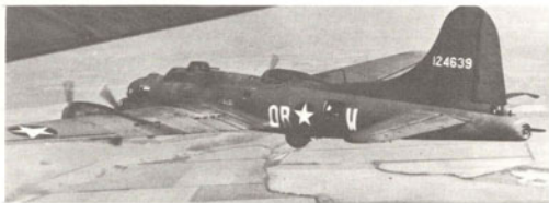
Upper surface view of the aircraft illustrated above showing position and size of National Insignia on wing. Code in white, serial in yellow. (USAF)
