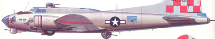
2 B-17G, 34th Bomb Group, 4th Bomb Squadron, ETO. White band and last three of serial in black on nose. Spring 1945.
