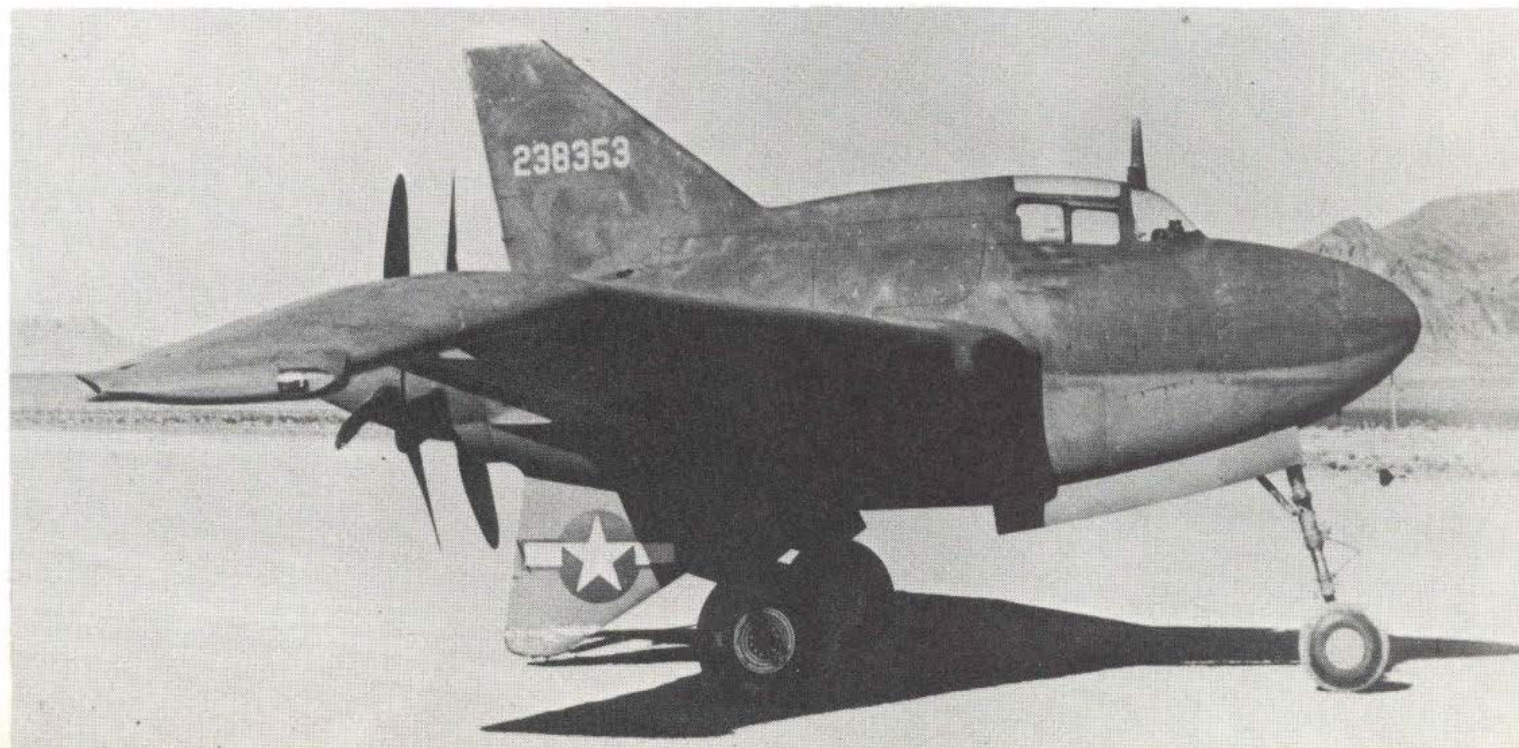
Below: Good detail shot of the 2nd prototype, note air-operated bellows rudders.
