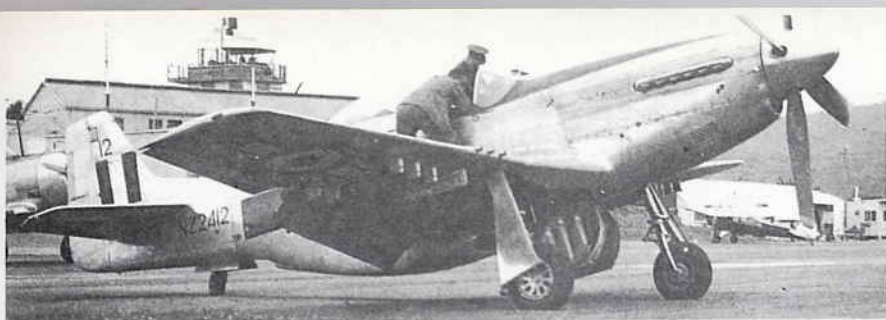
NZ2412, No. 3 Squadron. Note rocket attachment points. (d'E. C. Darby)
