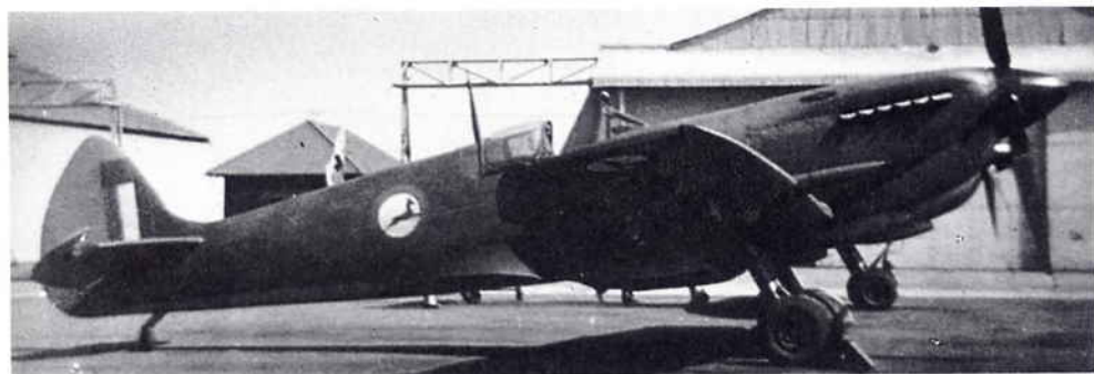
Mk. IXe, serial 5581. Note bomb and rocket attachment points. (SAAF)
