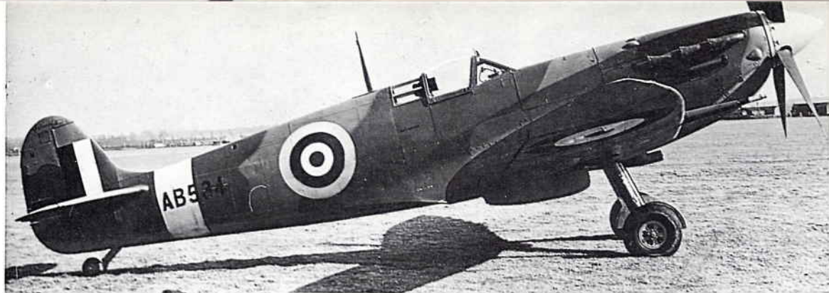
One of the less successful, and not so popular Spitfires was the Mk. VI. Note cabin pressurisation intake and extra frame on top of canopy, AB534 was later flown on No. 616 'South Yorkshire' Squadron in 1942 by 'Johnnie' Johnson. (HU2195 IWM)
