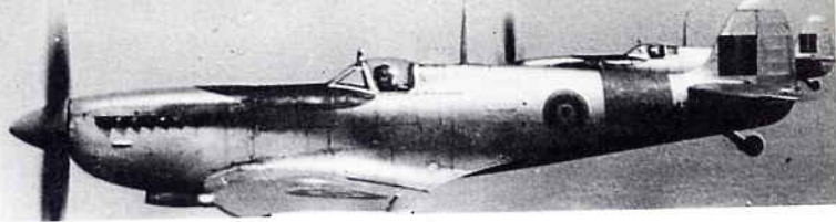
Mk. IX's of the Operational Training Unit, Brusthem, Belgian Air Force. Bare metal finish with black anti-glare panel, yellow fuselage and wing bands. Blue outline to national insignia. (via M. C. Terlinden)
