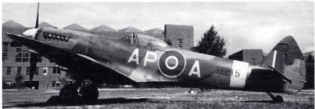
Above. While most Mk. IX aircraft did not have the 'tear-drop' canopy, a few late-production models incorporated this feature, as TE215, a HF IXe of No. 130 'Punjab' Squadron at Odiham in 1946. (via L. Bachelor)
