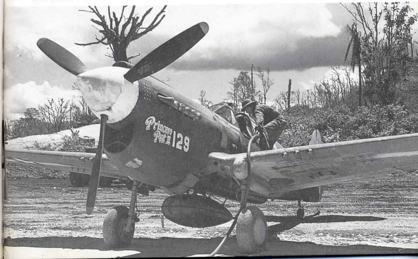
Above & below: P-40N 'Princess Pat II' being re-fuelled at Munda airfield. Note non-standard drop tank, 18th FG 44th FS. (USAF).
