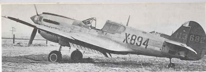
P-40R trainer (83rd P-40F re-engined). In natural metal with OD anti-glare panel, fin and rudder, red tip to spinner. (Peter M. Bowers).
