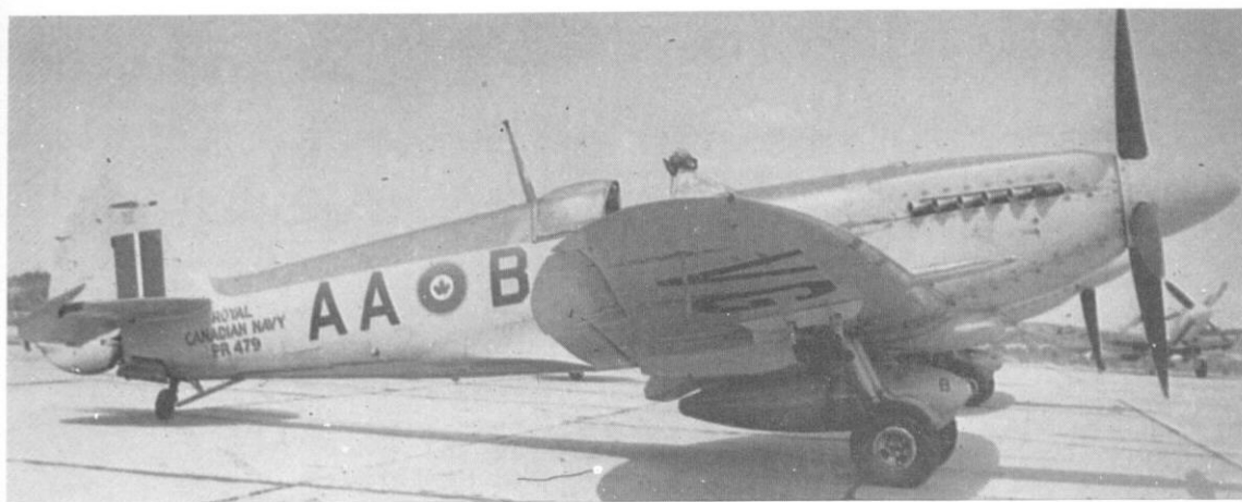
Above: Seafire F.XV, PR479, 1st Training Group, Dartmouth, Nova Scotia. The Canadian Seafires were unusual in having an aerial mast for H/T radio rather than the VHF 'whip' type. Note also the radio call-sign letters VG-AAB and its presentation under the wings and on the fuselage. (via F. G. Freeman Jr.).
