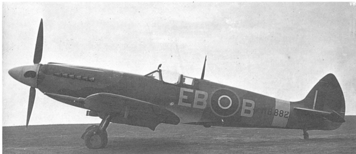
Good side view showing the new nose lines of the Mk. XII, MB882 of No. 41 Squadron. (IWM).
