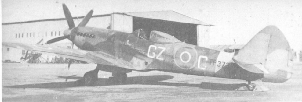
Above: FR XVIII, No. 32 Squadron in the Middle East, note the hunting horn insignia under cockpit. As seen on this and preceding photograph it was common practice to remove the oblique camera on FR type aircraft, the port being covered with fabric. TP373.
