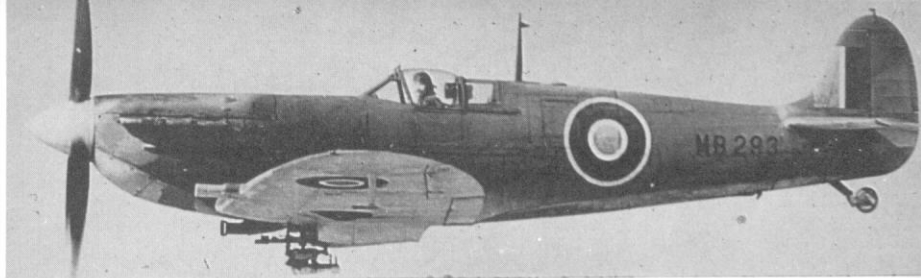
Seafire IIC MB293. The odd looking device under the fuselage is a trailing-static 'bomb' for calibrating airspeed during performance testing.
