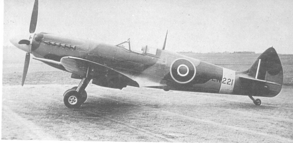
The first Spitfire Mk. XII, EN221. The wings were not clipped on this aircraft so that comparative tests could be run with EN222 which did have clipped wings. Both aircraft were flown by Flt.Lt. 'Spud' Potocki at the Intensive Flying Development Unit, Boscombe Down, December 1942.
