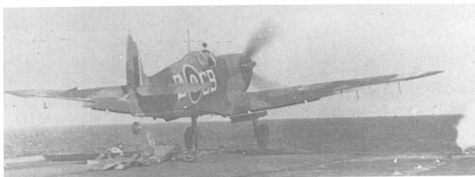
Seafire IIC of No. 885 Squadron, Ø6-B just leaving the catapult on HMS 'Furious' (D. R. Wheeler via D. J. Brown).
