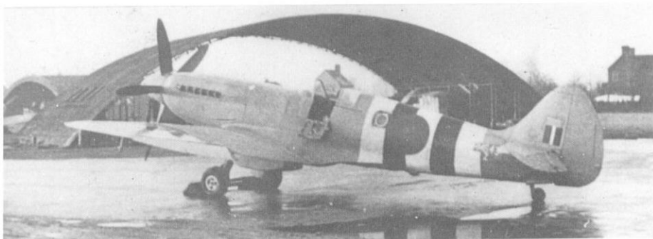
Above: One of the PR XIX's from the first production batch without pressurisation. RM645 is seen here with No. 682 Squadron, Italy, in early 1945. (via L. Bachelor).
