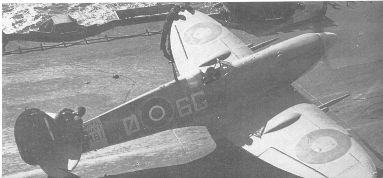
Seafire IIC MB156. No. 885 Squadron, HMS 'Formidable' well and truly held down whilst the engine is run up prior to take-off. (IWM).
