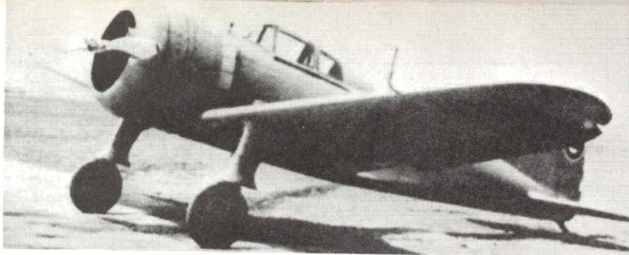
Left: The Ki.27a was modified for trainer use as the Ki.27a-Kai by removing the armament and wheel parts. The fuselage tail cone was frequently also removed. School markings are of the Kumagaya Army Flying School. (S. Abe via Bueschel).
