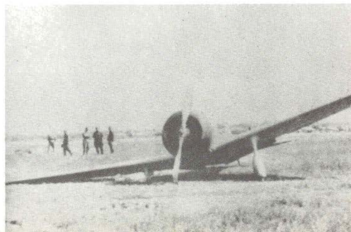
Below: A broken landing gear leg was an uncommon occurrence with the Type 97 Fighter as this aircraft was well designed and durable. (Sekai-no-Kokuki via Bueschel).
