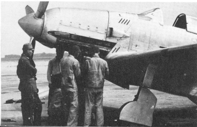
The Ki.60 differed externally from the parallel Ki.61 in having a snub nose, short moment-arm and shorter wings (M. Toda via Bueschel).
