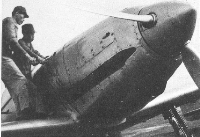
Kawasaki Ha.40 engine prototypes were not available for the Ki.60, so imported Daimler-Benz DB.601A power plants were used (Hideya Ando via Bueschel).
