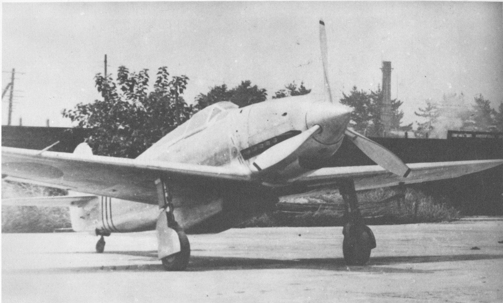
Prototype Ki.6003, last Ki.60 model to be built, had a top speed of 560 km/hr. Three red fuselage stripes denote Model 3 (Seiso Tachibana via Bueschel).
