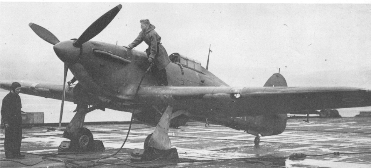
Below: Sea Hurricane Ib being serviced on a light carrier, note the cut-out for the arrester hook. (IWM)
