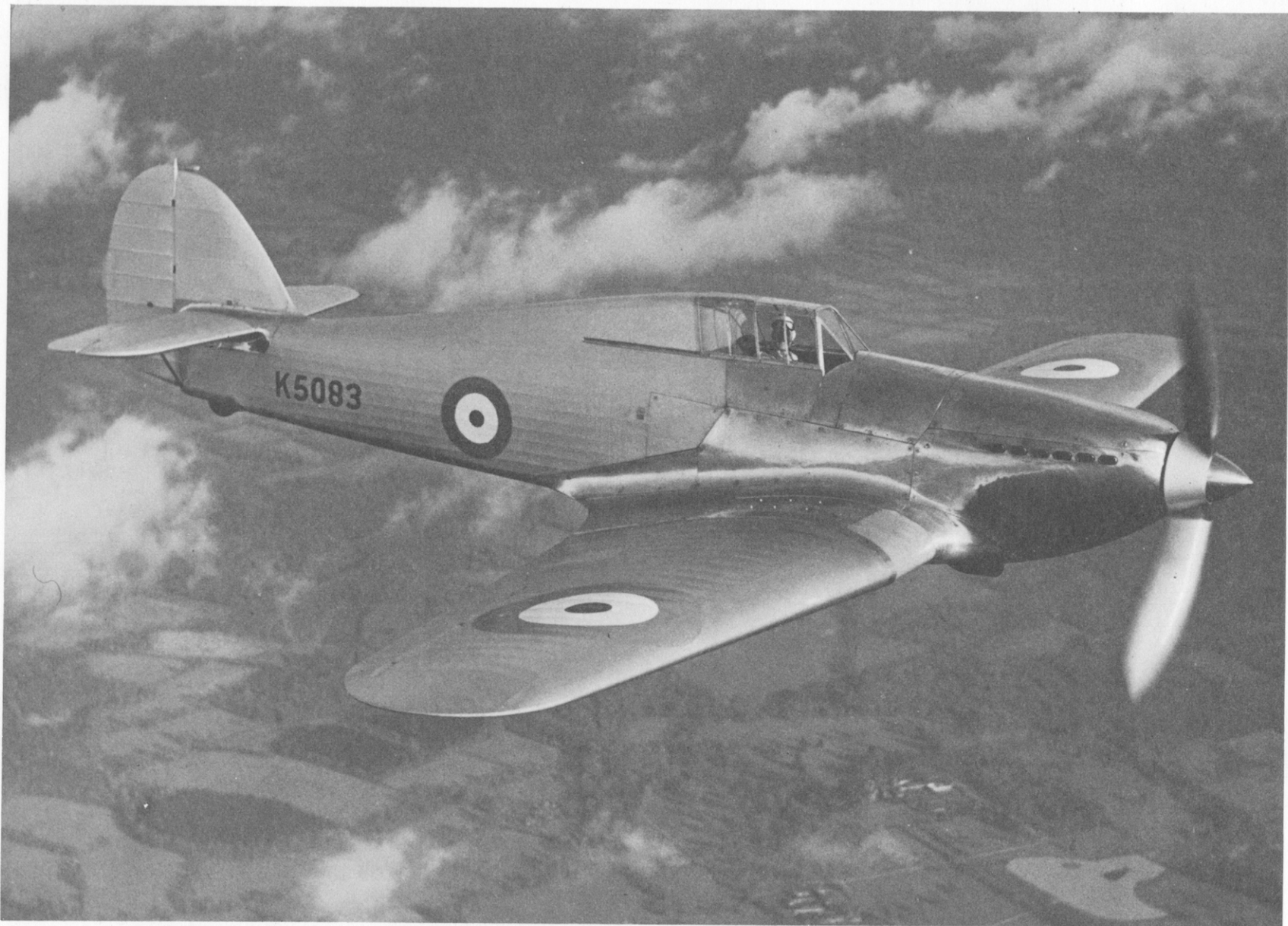
An early flying shot of K5083, the Hurricane prototype. This photograph was taken during flying trials before the fitting of the eight gun armament. (Hawker)
