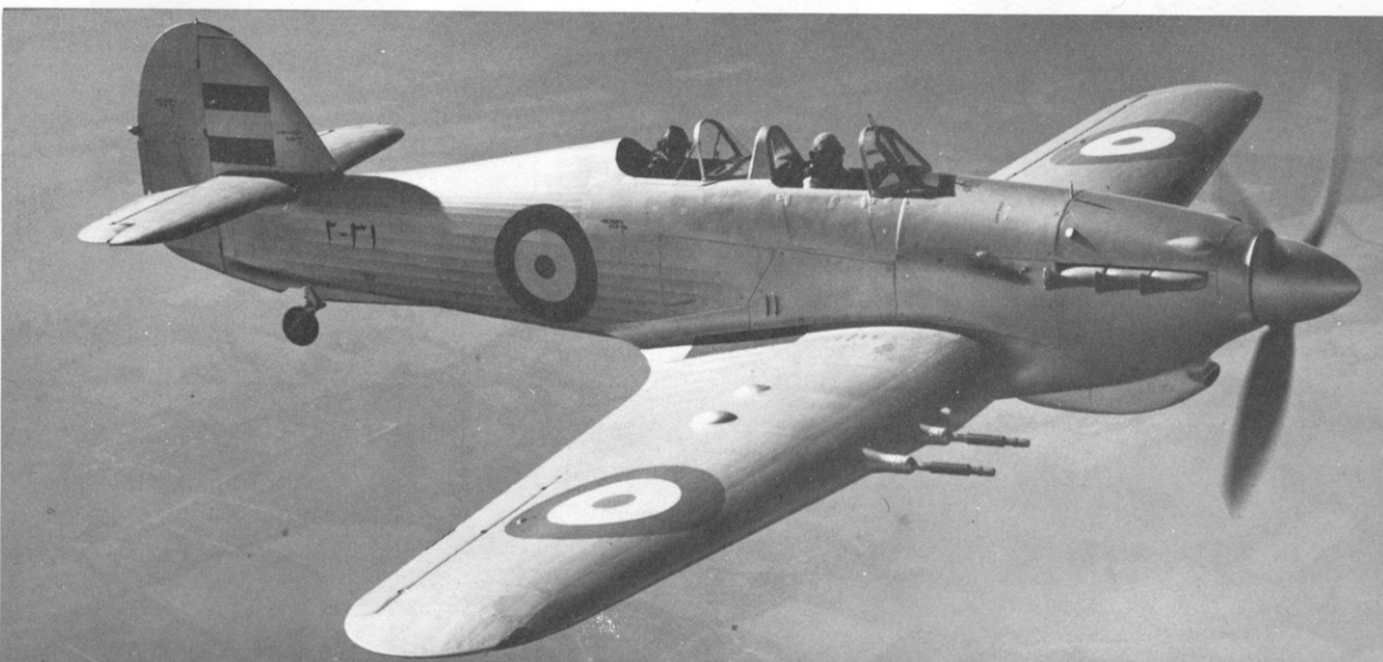
Below: Good flying shot of a Persian two-seater with early open cockpits and right, with the addition of a less draughty instructor's seat, a modified Tempest sliding hood. (Hawker)
