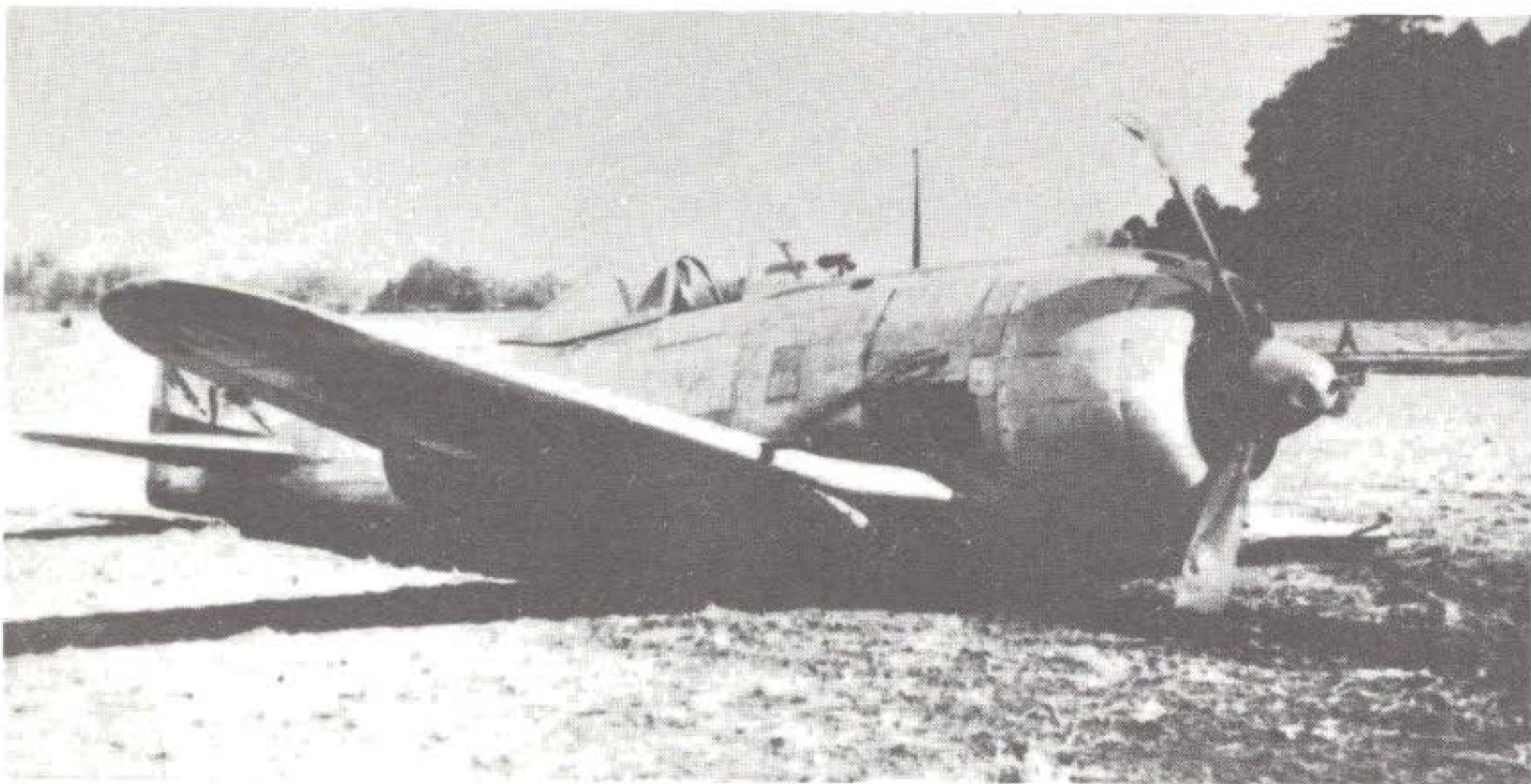
Wing guns are obvious on Shoki of 2nd Company, 47th Fighter Regiment. (M. Toda via Bueschel)
