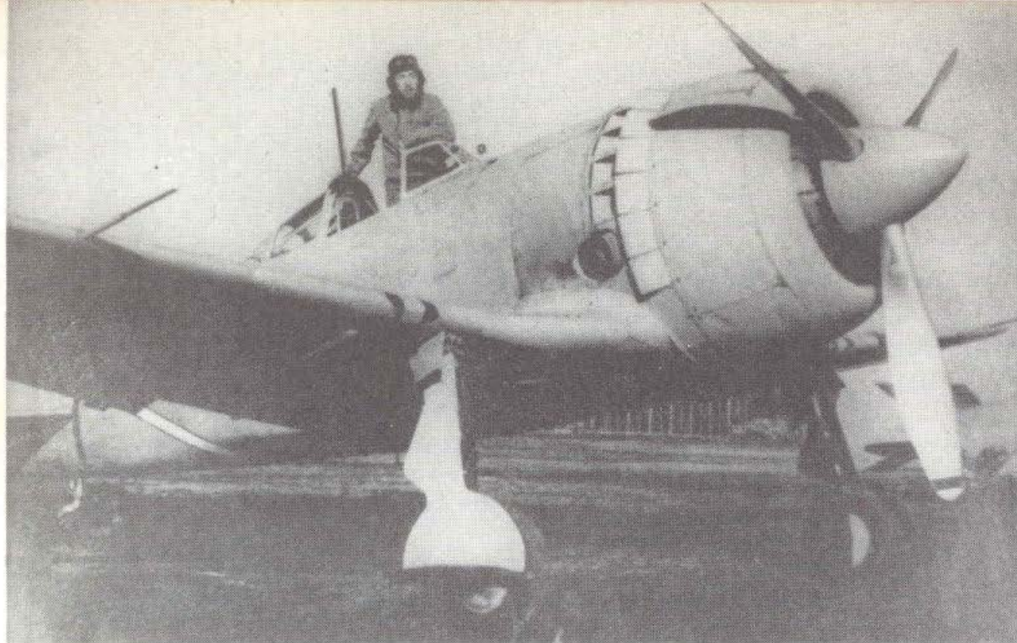
First prototype Ki.4401 completed in August 1940. Finish is Army grey-green with white and red stripes. Nakajima Ha.41 power plant exhaust vents circle upper cowl. (Koku Fan via Bueschel)
