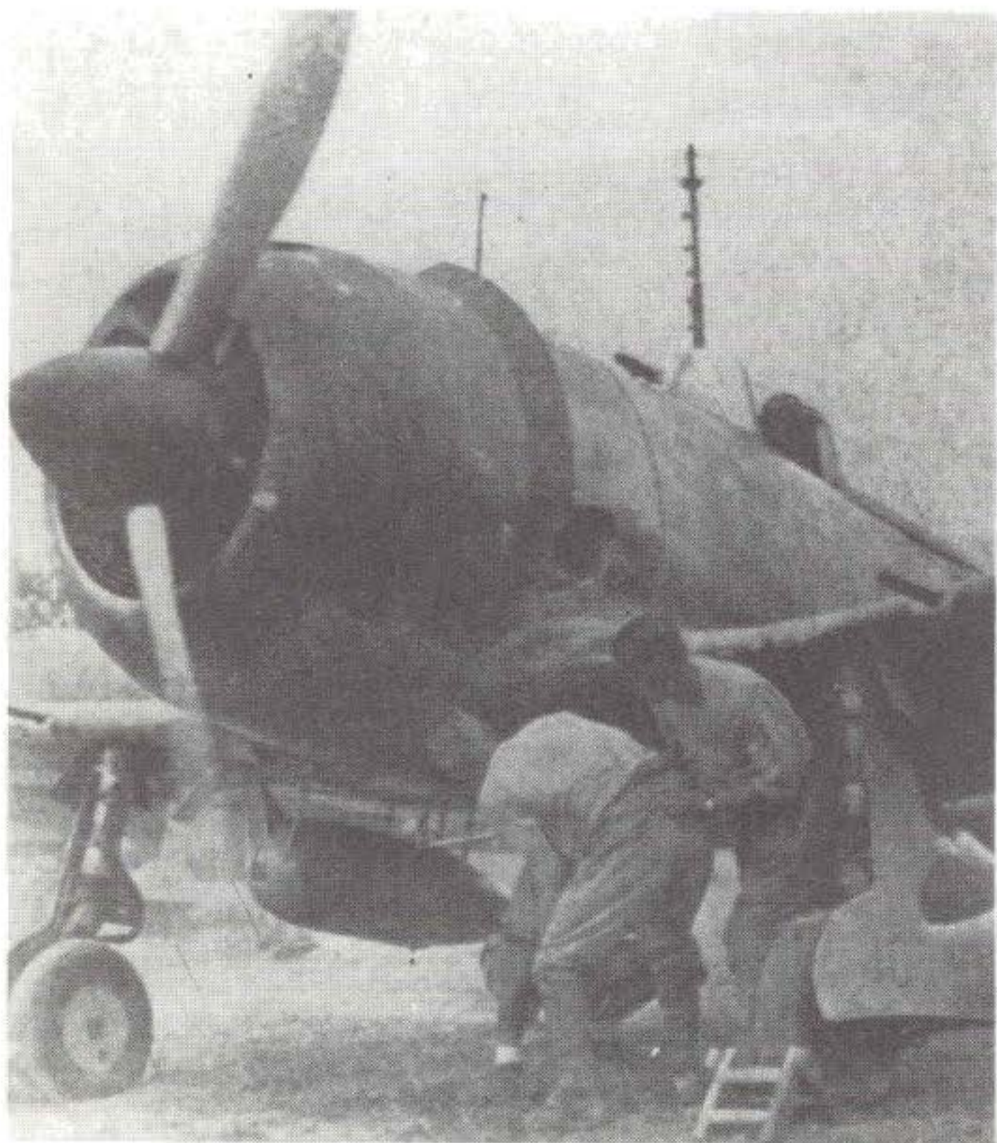
Pre-production prototype Ki.4410 of the 47th Fighter Company being readied for flight with dual drop tanks. (Koku Shonen via Bueschel)
