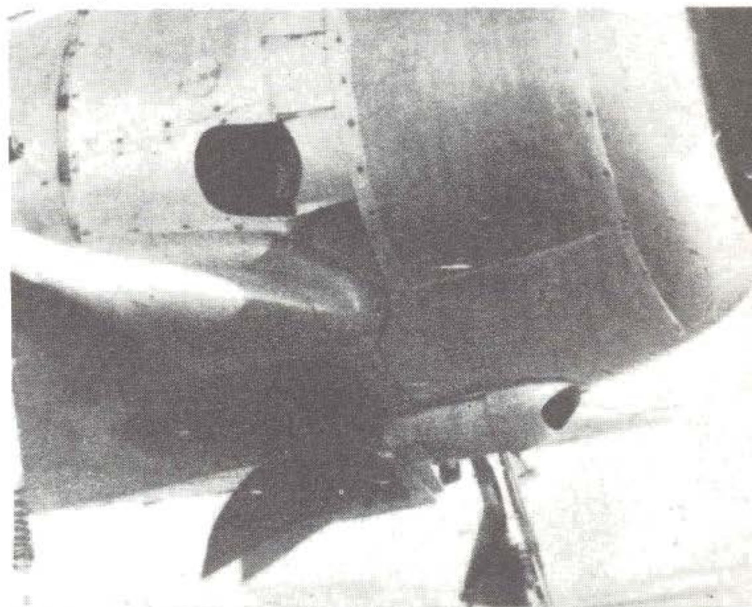
Oil scoop was an identification feature of Model 2. (Koku Shonen via Bueschel)
