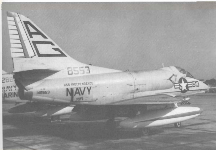
A-4C of VSF-1, USS Independence , 1969. Note 513 staggered on upper surface of starboard wing, repeated in white on flap face. (R. Harrison)
