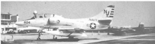
Below: Good detail shot of a TA-4E showing the modified and lengthened nose. (McDonnell-Douglas via J. W. R. Taylor)
