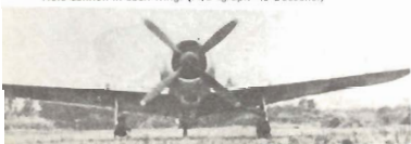
Below: Ki-84-Ia mounted 2 x 12-7mm Ho.103 guns in nose and a 20mm Ho.5 cannon in each wing. (Asahigraph via Bueschel)
