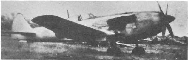
Below: Major difference from the Hayate design was the outboard landing gear of the Ki.87. (Nakajima Hikoki via Bueschel)
