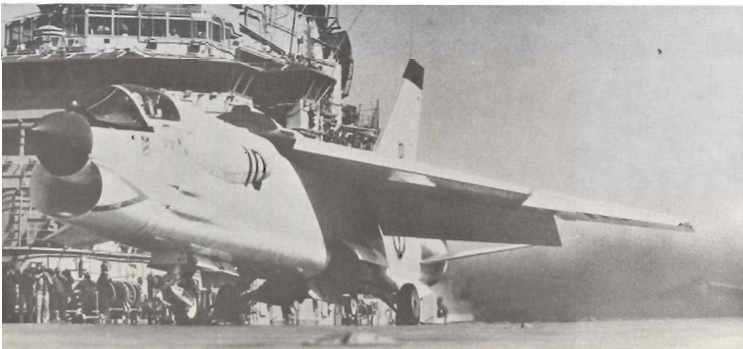
Below: Spewing black smoke out of its tailpipe, an F-8E(FN) Crusader runs up its J-57 in military power preparatory to being catapulted from the deck of the carrier Clemenceau . (Vought)
