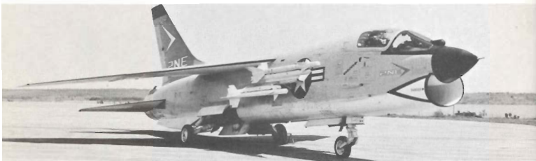
Above: F-8E with four Sidewinder I infra-red homing air-to-air missiles. (Vought) Below: F-8E armed with Zuni rockets and Bullbup B missiles. (Vought)
