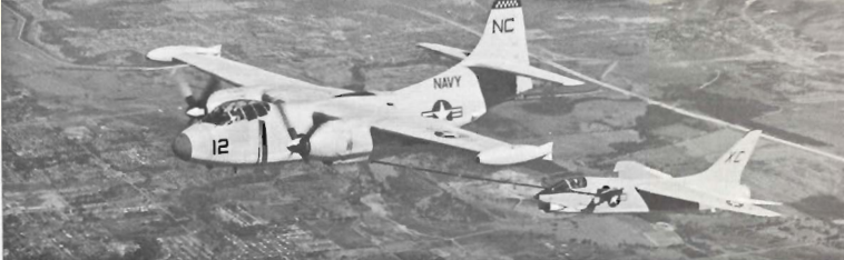
Above: F-8A of VX-3 being refueled by an AJ-2 tanker of VAH-11. (US Navy)
