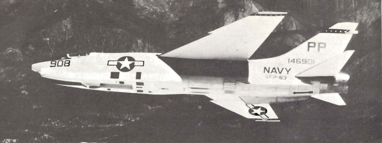
Above & below: RF-8G Crusaders of VFP-63, note the bulges on the fin of 900 containing tail snooping electronic gear. (US Navy)
