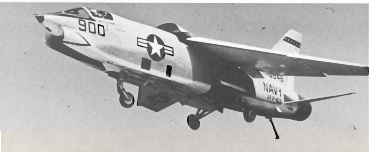
Below: An RF-8A Crusader coming in to land on the carrier USS Midway CVA-43 in the Gulf of Tonkin in late 1968. This view shows the matt black area from intake to camera housing and also the camera gun window in the nose cone. (US Navy via R. J. Francillon)
