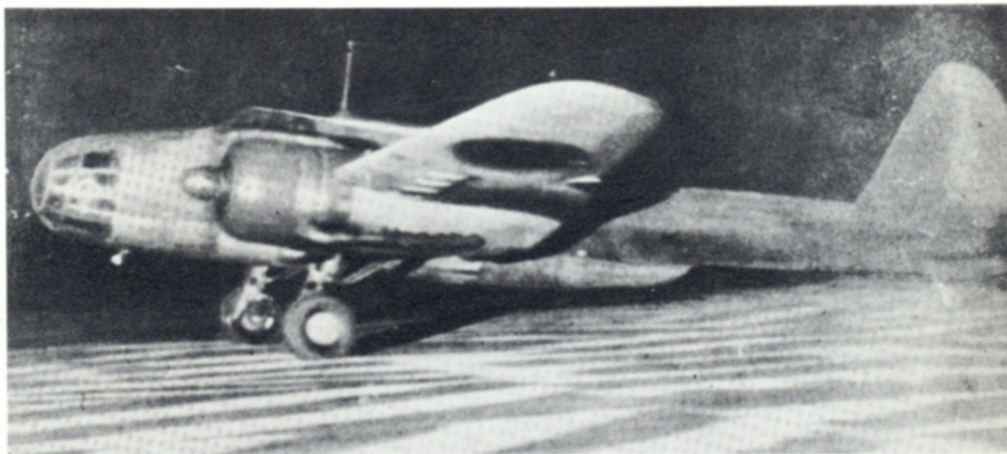
Below: Flame dampeners were fitted to exhausts for night operations in China. (Koku Asahi via Bueschel)
