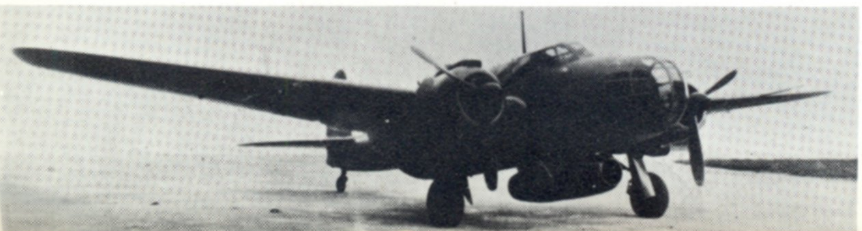
Below: Late 1943 experiment at Army Air Test Department at Fussa utilizes modified Ki.48-IIb as a test-bed for the Ne.00 turbojet. (Hideya Ando via Bueschel)
