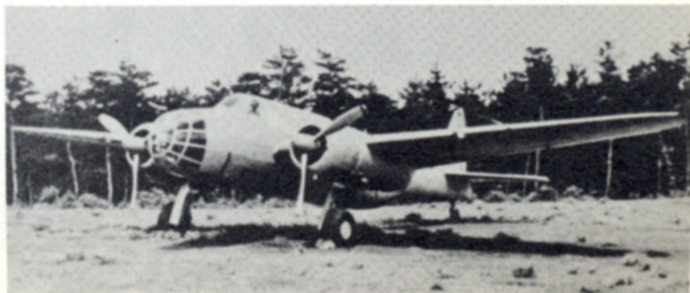
The next five prototypes, the first completed in September 1939, had a strengthened fuselage and redesigned tail section. The type was accepted for production in December 1939 in this form. (Sekai No Kokuki via Bueschel)
