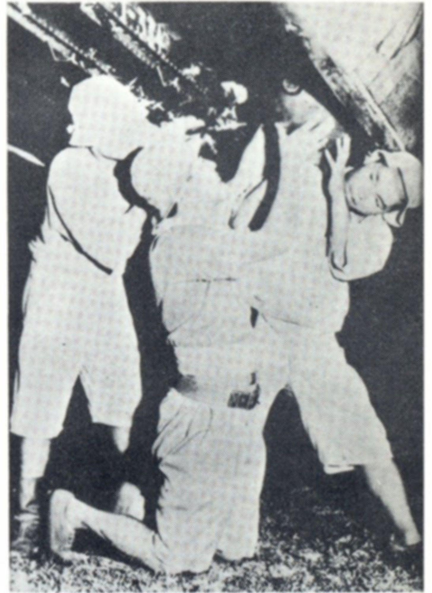
Above: Ground crewmen loading bombs into the narrow fuselage of the Ki.48-lb. (Warren D. Ship via Bueschel)
