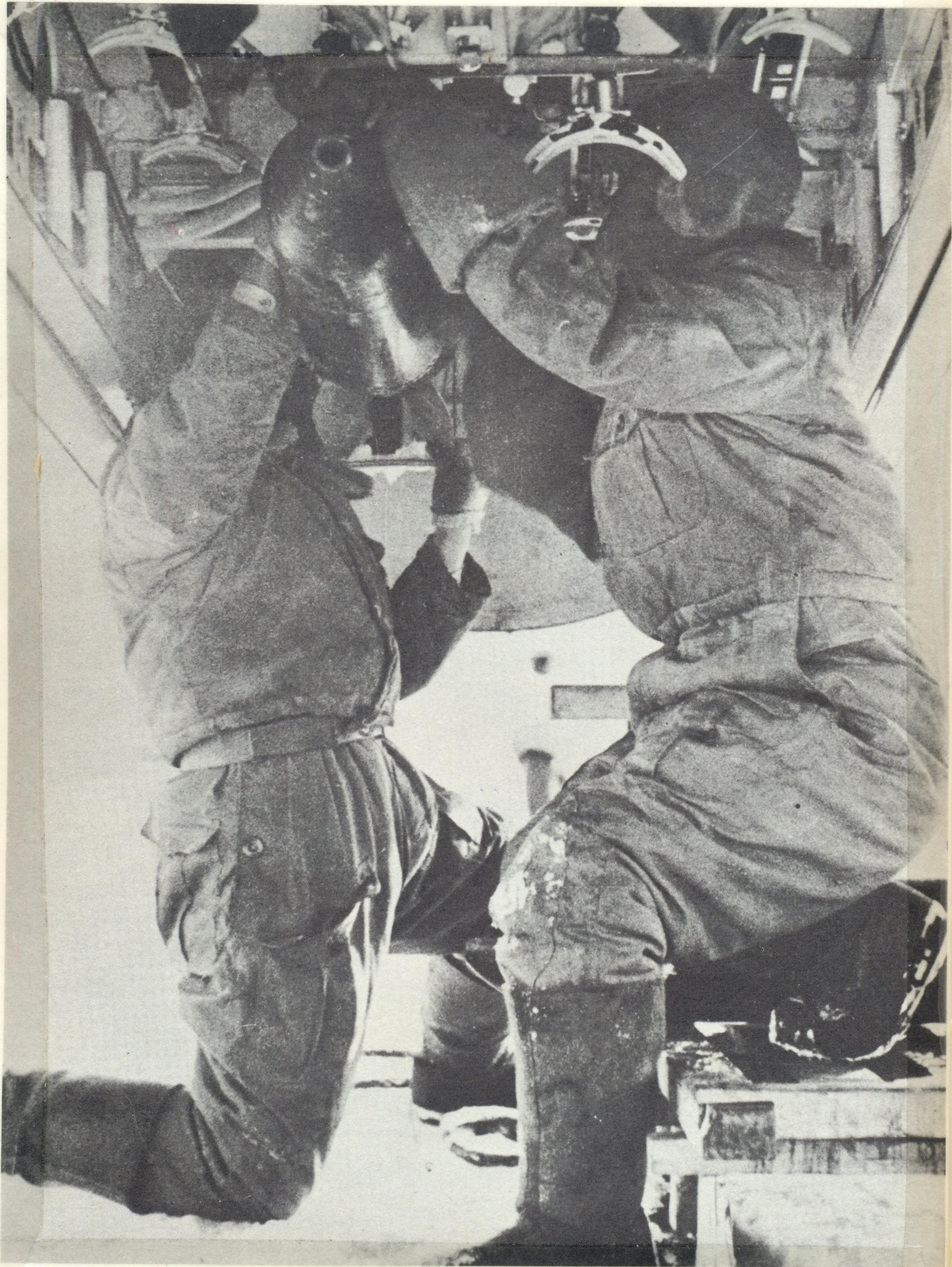
Standard load was six 100-pound bombs carried in internal racks. Alternate load was twenty-four 32-pound bombs. (Tohosya via Bueschel)
