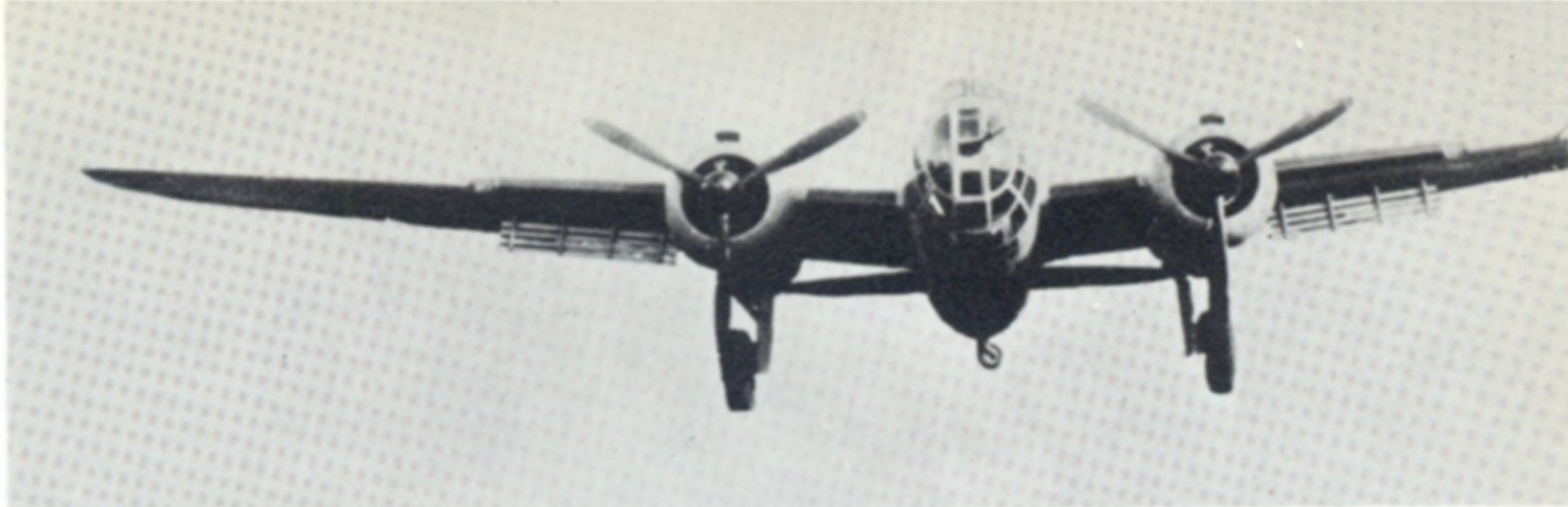
Above: Dive brakes were fitted to dive bomber prototypes. Some entered service where dive brakes were often removed to lighten weight. (Mannosuke Toda via Bueschel)
