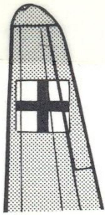
H3 Surrender marking, upper and under port and starboard.
