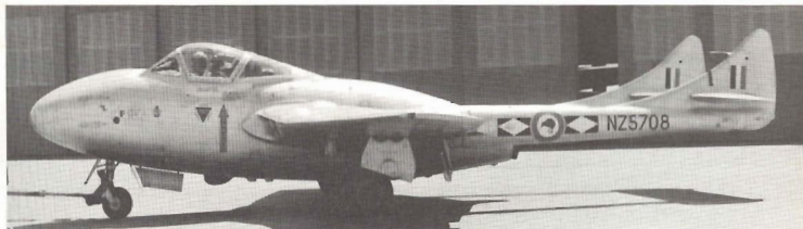
Above: T.11 of No. 14 Squadron, RNZAF. Note Kiwi on tail-boom roundels, yellow Rescue arrow, radome under fuselage. (RNZAF via D. A. Noble)
