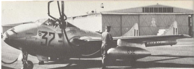
Above & below: Two of the 36 T.33's operated by the RAAF. Standard silver and orange dayglo finish, note radome under fuselage. (via R. C. B. Ashworth)
