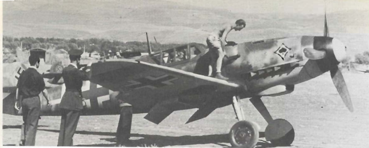
Above: a Bf 109G-6 of 6./JG 53 having the starter crank inserted and below a G-5 equipped with Wfr.Gr.21 mortars and belly tank.
