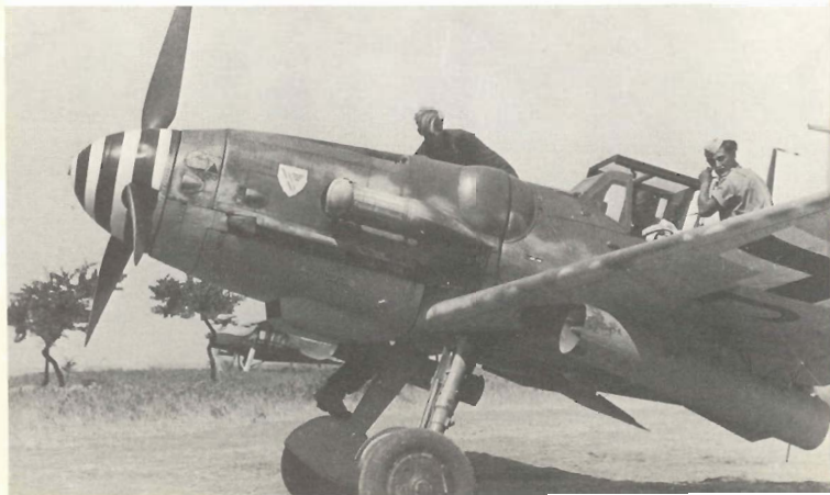
Below: A Bf 109G-6/R2 Trop of III./JG 3 "Udet" armed with Wfr.Gr. 21 mortars beneath the wings.
