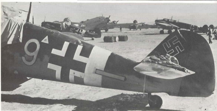
Above, both pictures: Yellow 9 showing nose and tail detail, European camouflage, no thin black line to under-wing and fuselage crosses, upper-wing crosses white outline only, see bottom photo on preceding page.
