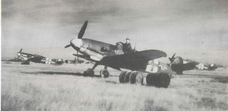
Fine photograph of Bf 109G-2's of III./JG 54 "Grünherz" on a Russian airfield during the summer of 1943. The under surface yellow extends to the black cross on the nearest aircraft and the upper surface scheme is standard black and dark green with grey areas added.
