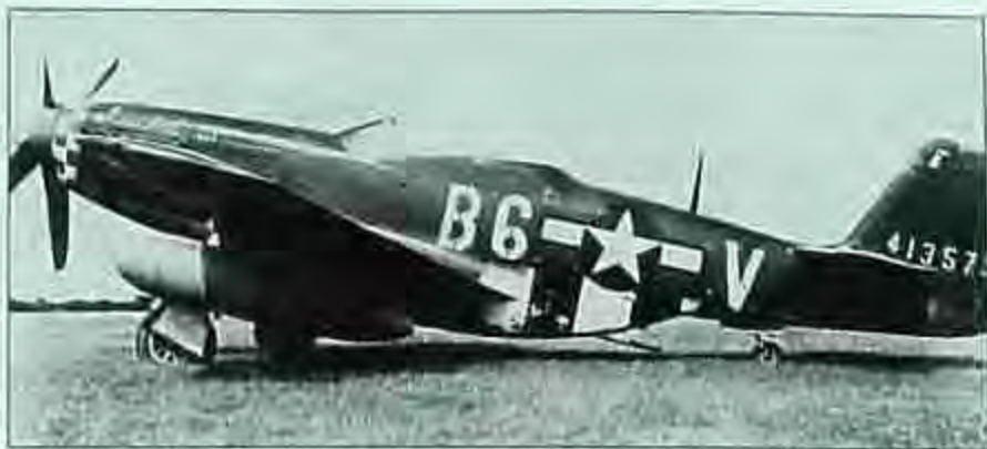
Early P-51D-5s lacked the dorsal fin fillet, as 44-13573 of the 357th FG's 363rd FS clearly shows. Although this sub-type successfully flew numerous combat missions, fillets were sent to the UK by NAA for adoption as 'field modifications'. The dorsal appendage was designed to correct minor directional stability problems encountered with the P-51B. Isabel III wears two victory crosses under its windscreen (Via T R Bennett)
