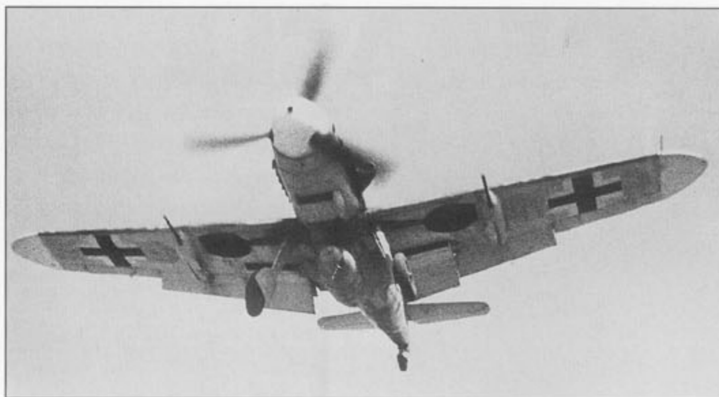
Fine detail view of the 'Kanonenboot's' twin 20 mm guns that gave the Bf 109G-6/R6 a very useful increase in firepower. Still fitted with its belly tank, this JG 53 fighter was photographed returning to its Tunisian base following an uneventful sortie in early 1943 – a rare event at this point in the campaign
