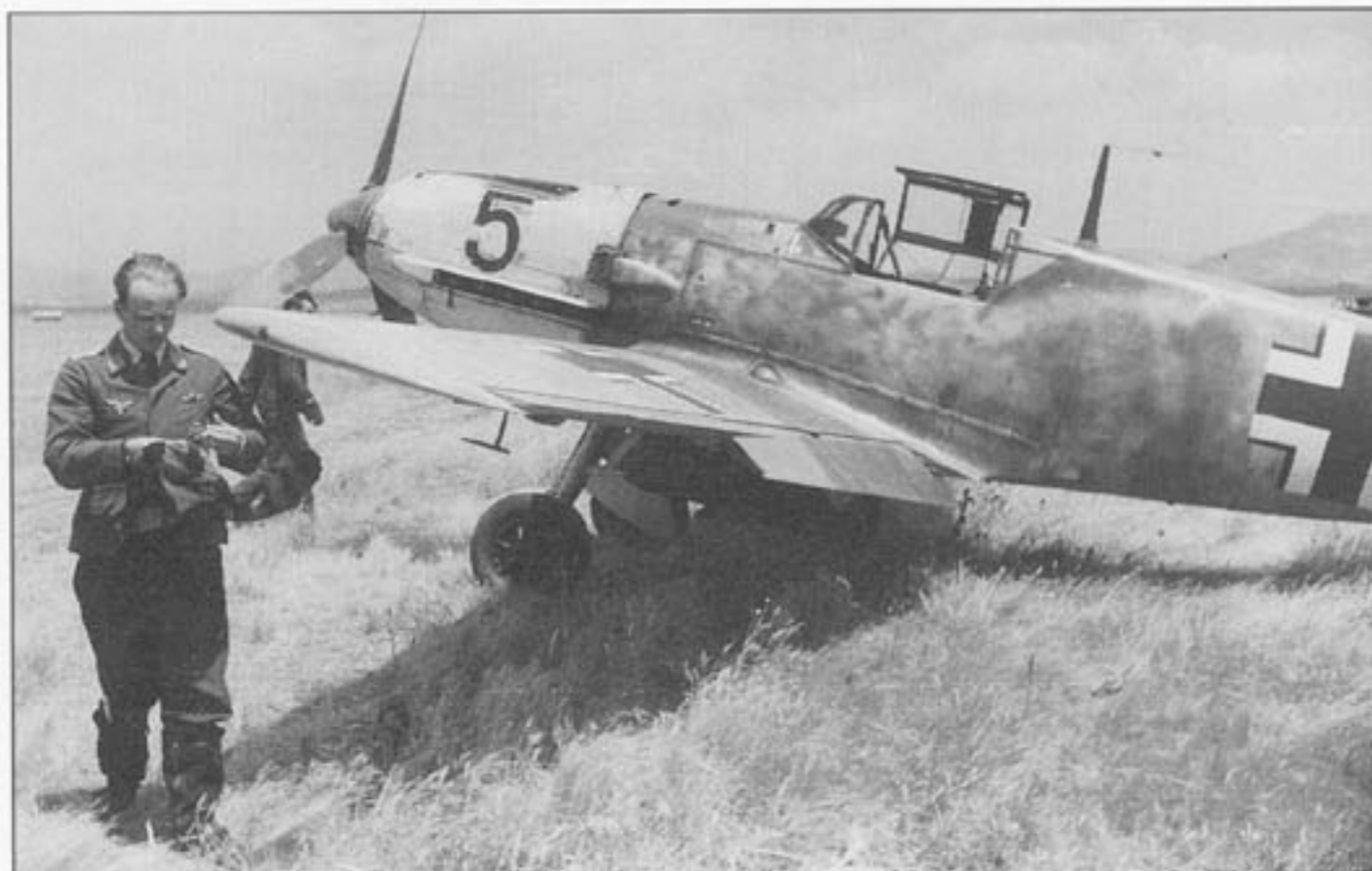
The island garrison of Malta was attacked by both fighter and Jabo Staffeln , the latter being deployed by 8./JG 27. Bf 109E-7 'Black 5' of this specialist fighter/bomber unit is seen here in May 1941 fully bombed up with a single SC250 device fitted to the centreline SC500 stores rack
