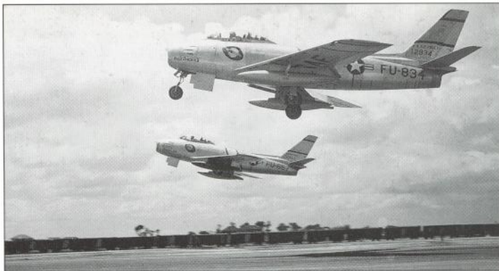
F-86s of the 336th FIS 'Rocketeers' launch from Kimpo airfield for a combat sweep along MiG Alley. In the foreground is a North American F-86E-10-NA (51-2834, UNCLE DOMINICK II ) and behind it a Canadair F-86E-6-CAN (52-2857), one of 60 fighters produced for the USAF in Canada. The E-model Sabre introduced an 'all-flying tail' which enhanced manoeuvrability and narrowed the gap in performance with the MiG-15. After the first year of the Korean War, the 4th FIW wore yellow bands on its Sabres, and was distinguished from other fighter wings by having the yellow band also emblazoned in the fin of its aircraft ( Sherman Tandvig )
