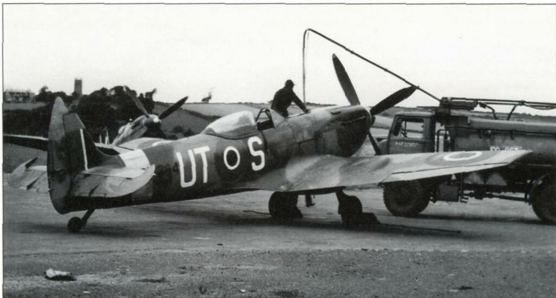
This view of a Spitfire Mk XVI of No 17 Sqn refuelling at Seletar in September 1945 clearly shows the size of the 'bubble' canopy, as well the degree of cutback built into the rear fuselage by Vickers-Armstrong. Based in the Far East from mid-1942 through to VJ Day, No 17 retained their Mk XVI's until they returned to the UK in 1948
