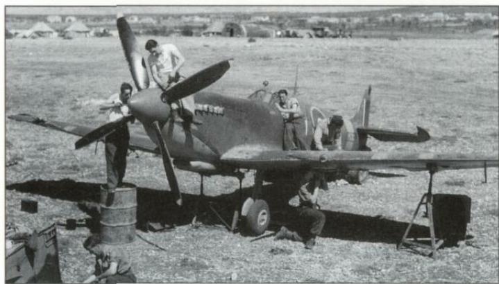
This Spitfire Mk VIII of No 253 Sqn has clipped wings, a fit rarely observed on the Mk VIII despite it being a common mod on other marks of the Supermarine fighter. Here, it is seen undergoing basic field servicing at Prkos, Yugoslavia, in early 1945 (via Bruce Robertson)
