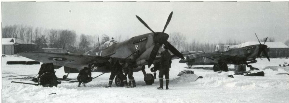
Two Mk IXs from No 317 'City of Wilno' Sqn are bombed up and plugged in to their respective acc trolleys in preparation for a short-notice scramble from Grimbergen in January 1945 (via Jerry Scutts)
