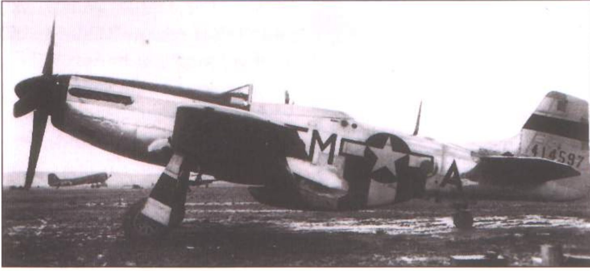
John Hoefker's F-6D 44-14597 sits amongst the puddles at a damp St Dizier airfield in France in late 1944. A camera port can just be seen cutting into the fuselage 'star and bar'. The 15th TRS refrained from adopting garish unit markings until well into 1945, as '5M-A' clearly shows ( Hoefker via Ivie )
