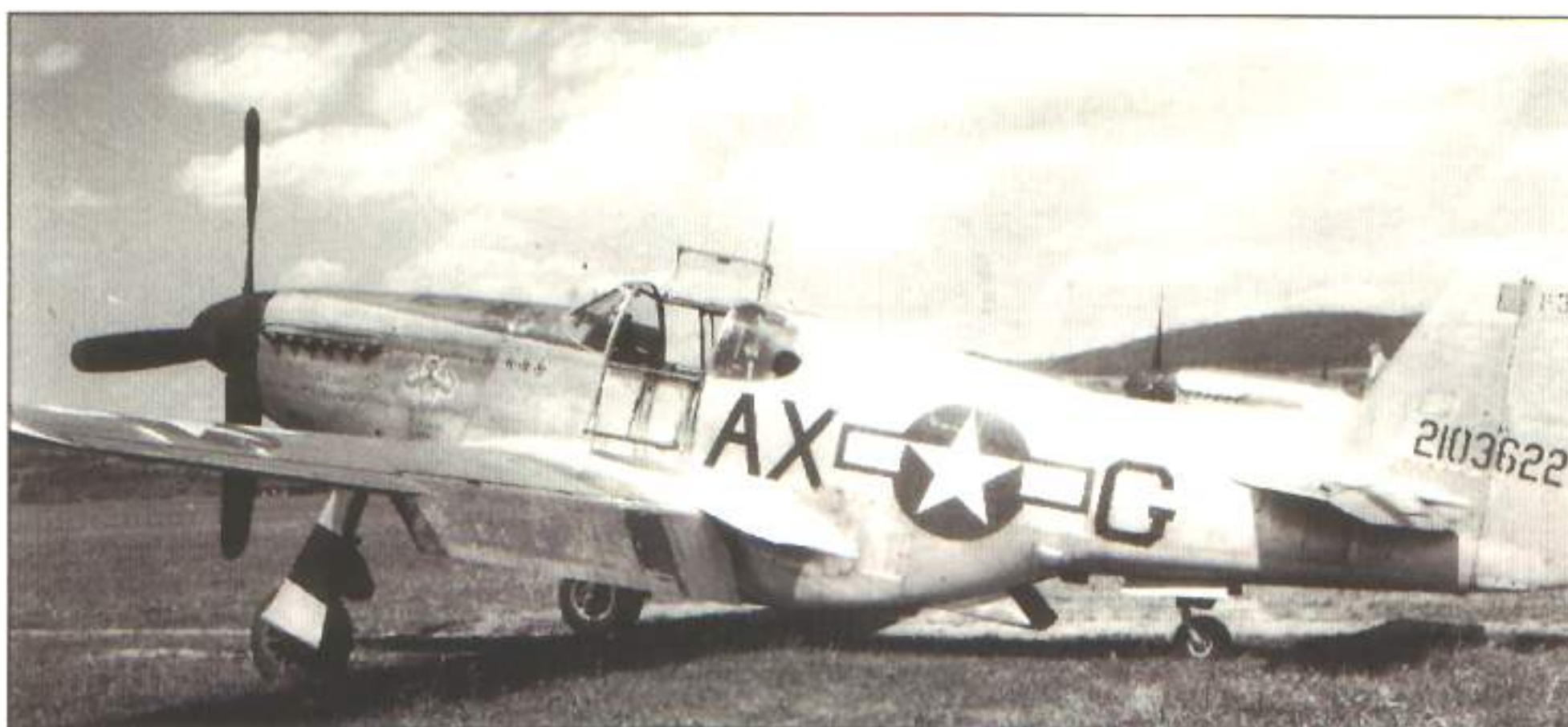
An F-6B of the 107th TRS/67th TRG, the AAF unit that first operated a version of the Mustang in the ETO. Going operational with the F-6A in October 1943, the 67th therefore beat the 354th to this distinction by about two months. And that its aircraft were flown fully armed with both cameras and guns is clearly demonstrated by the three kills marked on 42-103622 ( Olmsted )
