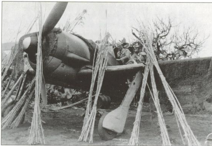
An Fw 190 of II./JG 2 hides behind some rudimentary camouflage at Tindja-South late in 1942. Note the dark appearance of the upper surfaces compared to the undersides. Witnesses have stated that the Gruppe's aircraft wore a fresh coat of unfaded tan overall at this period. Leutnant Gehr, standing beside the cockpit in tropical uniform, is camouflaged even more effectively against a background of cactus!
