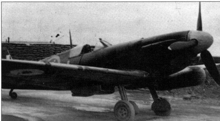
Spitfire IIA (long range) of No 118 Sqn shows off its 40-gallon fixed tank under the port wing whilst parked at Ibsley in April 1941. This modification was initially trialled on the Mark I ( Lambertmont )
