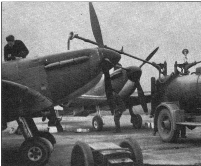
Spitfires of No 66 Sqn drawn together for rapid refuelling at Duxford in early 1940. Once the Fighter Command airfields came under threat of attack, aircraft were dispersed and refuelled individually so as not to offer such an inviting target
