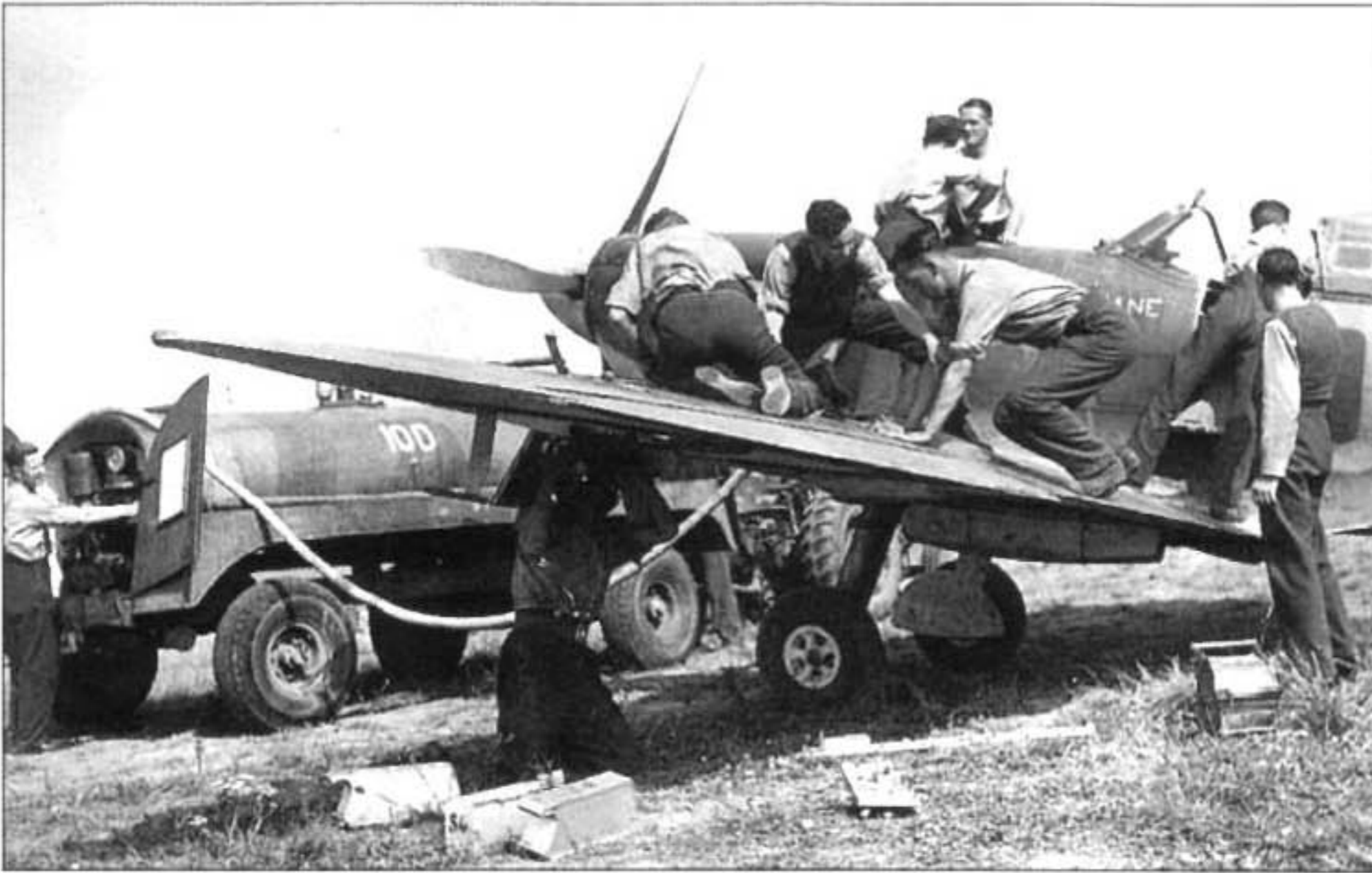
Groundcrewman swarm over a Mk VB of No 485 'New Zealand' Sqn at Redhill in August 1941, carrying out a rapid refuelling and re-arming between sorties. Note the partially empty boxes of .303-in ammunition in the centre foreground, and the 20 mm drum magazine at the right foreground ( via Scutts )
