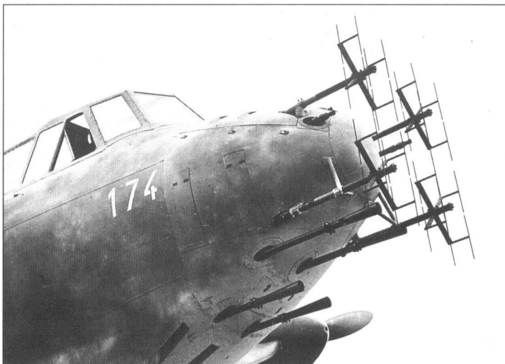
This close-up shot shows the complex arrangement of FuG 202 aerials, four MG 151 20 mm cannon barrels (fitted with flash suppressors) below the antennae and four MG 17 machine guns above which crowded the nose section of the Do 217N-2. This combination made the converted Dornier bomber a formidable opponent once it started appearing in the night skies over occupied Europe during the winter of 1942/43 (Aerospace)
