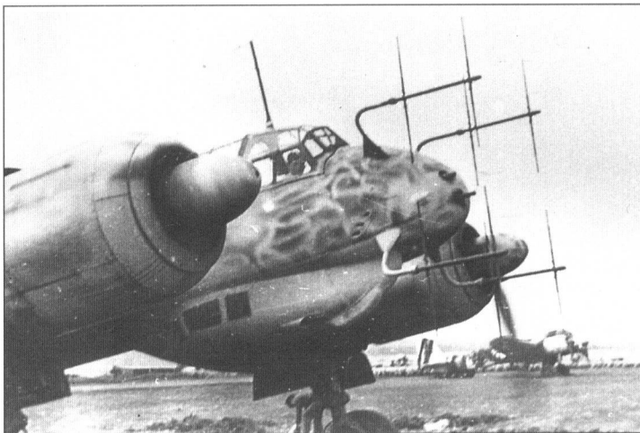
A close up of a Ju 88R-2 reveals its BMW engines and an early style gondola, which was dispensed with on the G-series. The SN-2 radar aerials seen here are as 'clean' as they ever got, with strengthened mounting sections at the base of each 'antler' in this instance (Creek)
