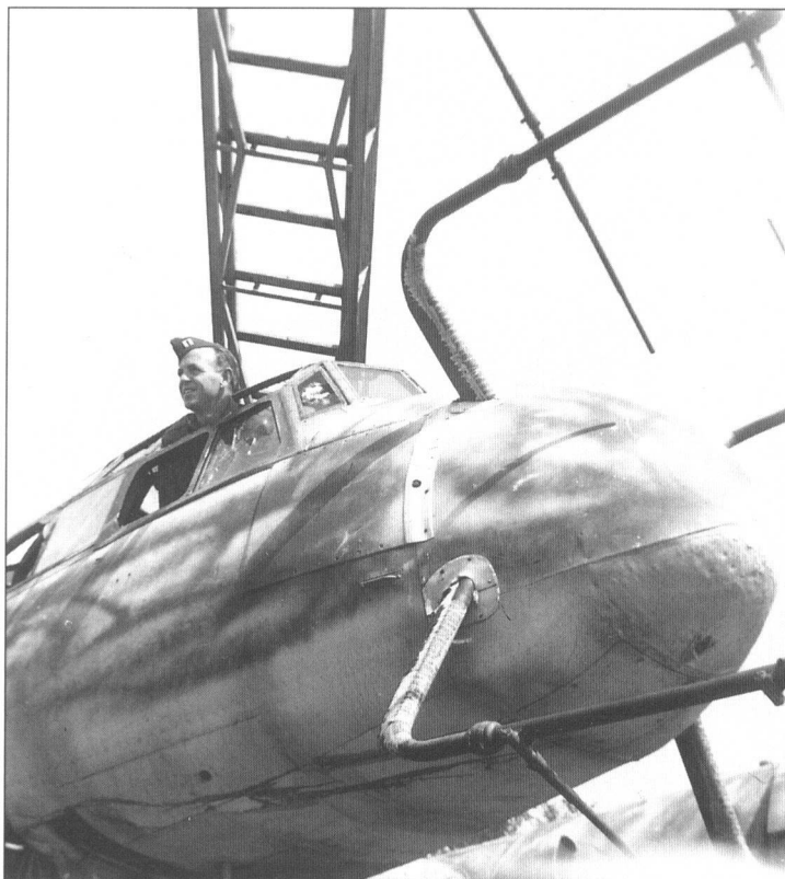
'Ribbed' base sections are in evidence in this close up view of the anchorage posts for the SN-2 aerials of a Ju 88G-6 captured by US forces (Crow)
