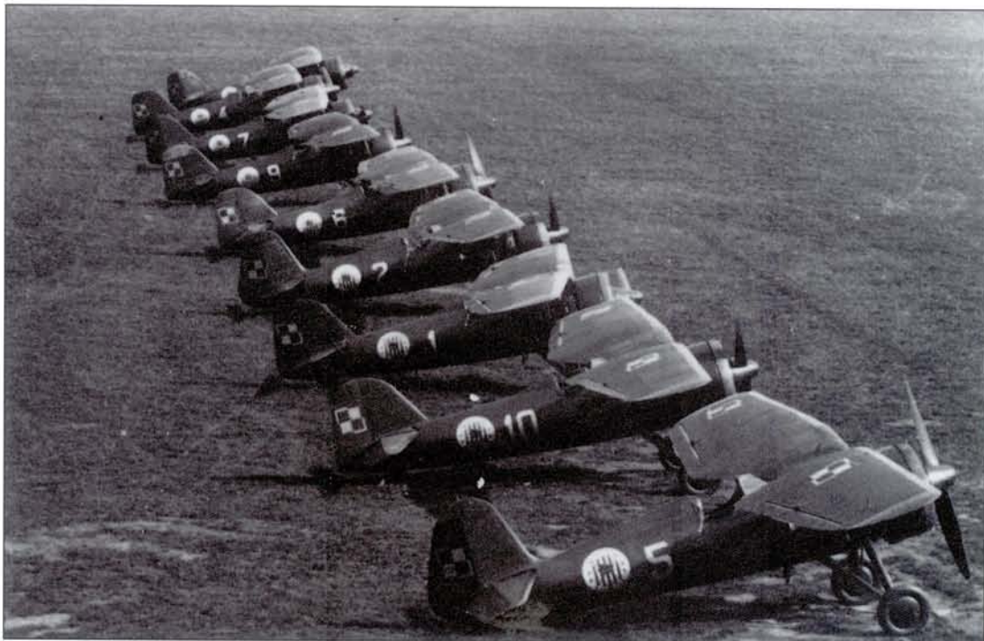
Fighters of 111 Eskadra . This unit inherited the Kościuszko tradition, and continued to use the 1920-vintage badge. In this view (probably taken during the weeks prior to the outbreak of war), 'White 5' and '1' are P.11cs, while the remaining aircraft are older P.11as ( Kopański )
