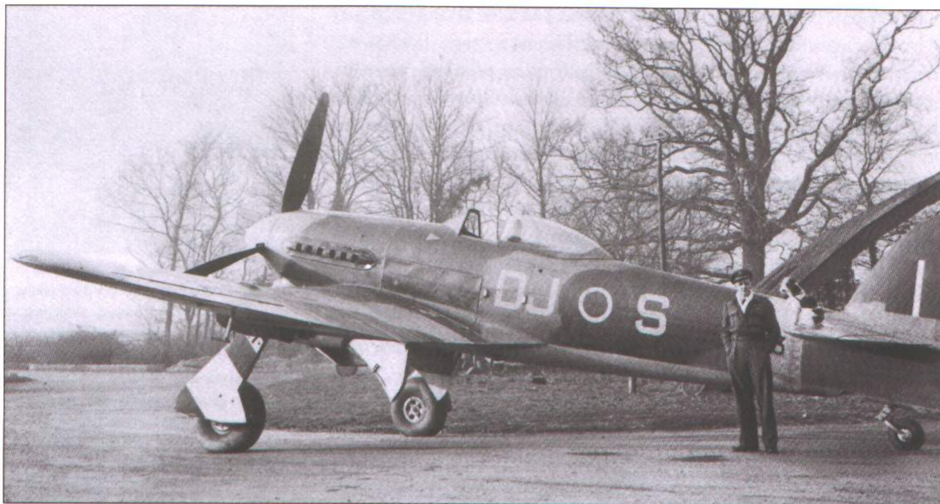
Promoted to lead the Tangmere Wing, Wg Cdr Des Scott is seen posing alongside his Typhoon, R8843, which carried his initials. This was the first Typhoon with the sliding hood, which did so much to improve visibility from the cockpit, to reach an operational unit. Supplies were slow at first, and such aircraft remained the privilege of squadron and flight commanders on most units well into 1944 (D J Scott)
