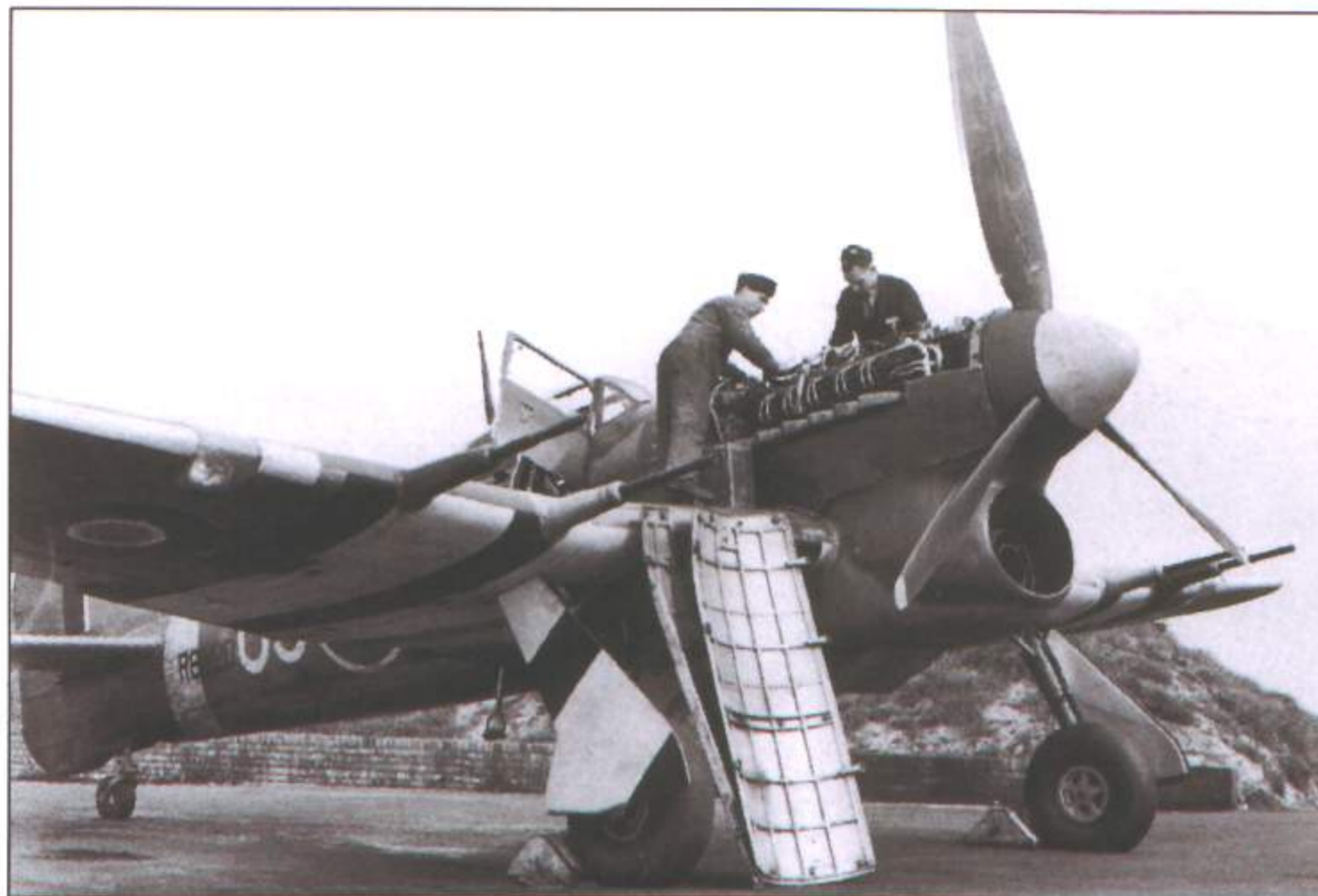
Photographed on the same occasion as the previous aircraft, R8220 'US-D' (another Hawker-built machine) is seen with its engine cowls removed and fitters working on the Sabre engine. Half obscured by the fitter's leg is a badge showing a diving Typhoon, marked 'US-D', shattering a swastika and captioned 'Shape of things to come'. Note the yellow leading edge stripe terminates just after the outer cannon ( Aeroplane )
