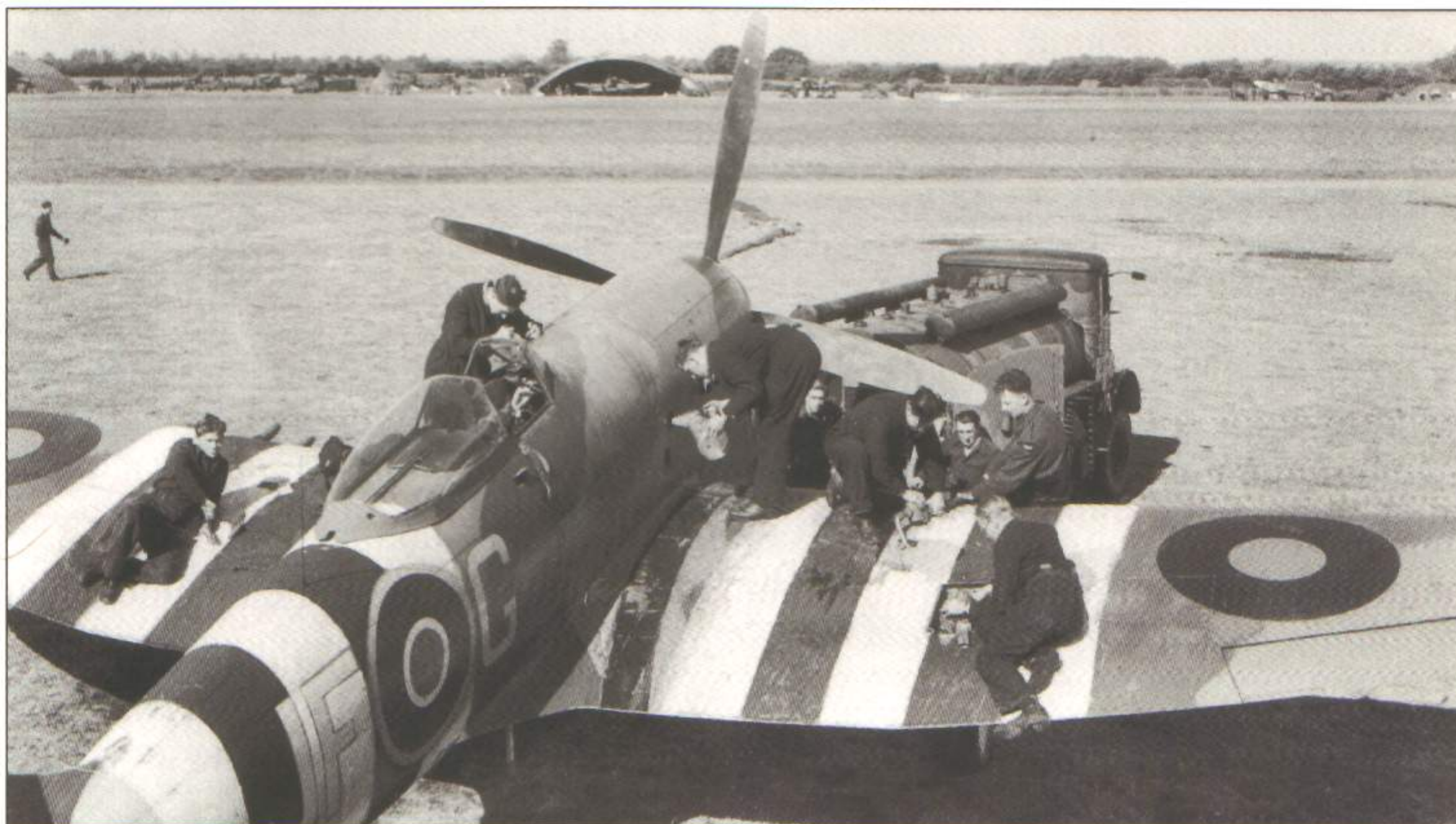
Quick turn-arounds were the order of the day at Newchurch so as to maintain the level of anti-'Diver' patrols required. On the starboard wing refuelling is taking place, while an armourer tends to the ammunition bay and an engine fitter tops up the oil (IWM CH 14088)
