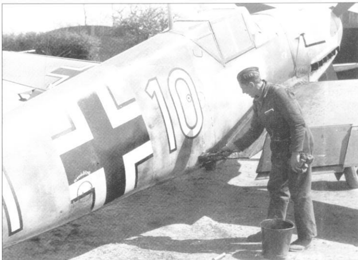
A III./JG 26 'black man' (Luftwaffe slang for groundcrew, so called because of the colour of their overalls) is seen busily engaged in removing the accumulated exhaust and oil stains before 'White 10's' next flight – note the starting handle already in place
