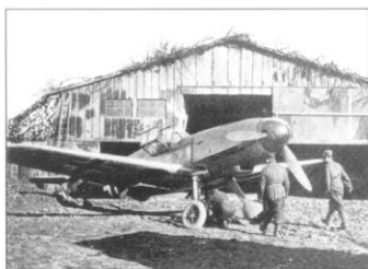
Parked outside a camouflaged hangar, this yellow-cowlinged Bf 109F is having its undercarriage worked on
