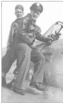
Wielding a screwdriver, Mel Paisley removes the radio panel cover plate from La Mort . This plate was simply screwed onto a pilot's newly-assigned P-47 soon after it was allocated to him, thus saving the groundcrew from having to paint the names on the replacement aircraft. This practise extended to exchanging full engine cowling panels if the nose-art was particularly well done, or if the pilot had paid good money to have it rendered ( Paisley )
