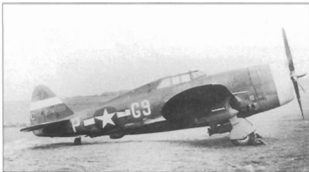
The 405th FG, based at nearby Christchurch, in Hampshire, 'loaned' one of its Thunderbolts to the Aircraft & Armaments Experimental Establishment (A&AEE) at Boscombe Down during the spring of 1944 to allow the P-47 to trial British, rather than American, ordnance. Here, the aircraft in question (P-47D-6 42-74599 from the 509th FS) is seen carrying the short, round-finned British bombs on its wing and belly racks. There were several Thunderbolts at the A&AEE at that time, and it is believed that these tests were part of a programme anticipating RAF use of the P-47 in the Far East later in the war. Note the fairly common application of the flight letter to the trim tab of this aircraft (via Tim Mason)
