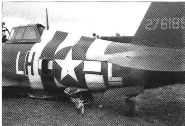
Yet another battle-damaged 353rd FG Thunderbolt, P-47D-15 42-76189 struggled back to Metfield, where its pilot carried out a textbook belly landing. This photograph reveals that the D-Day invasion stripes applied by some groups to their aircraft passed right around the fuselage. The turbosupercharger unit fitted in the underbelly of the P-47 also appears to have been partially ripped away by the impact of the landing
