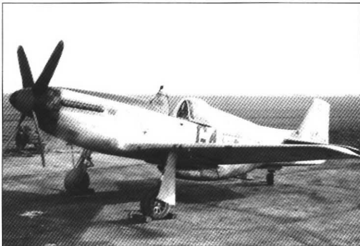
P-51B-10 43-7184 of the 362nd FS/357th FG features several modifications to the standard production aircraft. Firstly, it has a Spitfire rear-view mirror, secondly, a 'Malcolm hood', and thirdly a dorsal fin – the latter modification was rarely seen on B-model Mustangs (via Michael O'Leary)
