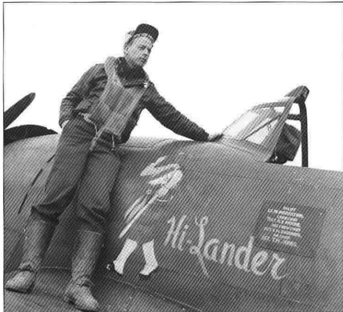
The 352nd FS's Lt Mike Morrison poses alongside his uniquely marked P-47C Hi-Lander at Metfield in late 1943. Note the cover on the gunsight, the rear view mirror and the complex structure of the early Thunderbolt windscreen (via Michael O'Leary)
