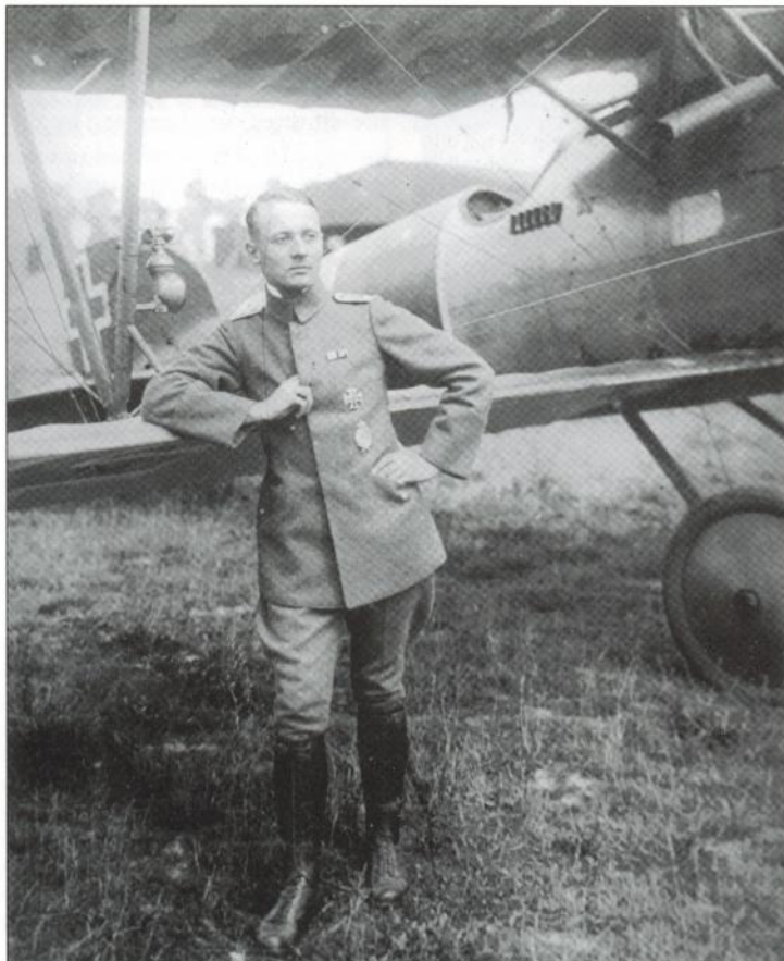
Friedrich 'Fritz' Ritter von Röth led Jasta 16b following service with Jasta 23b . He is leaning on an Albatros D Va that features the black tail unit of Jasta 16b , as well as a coloured fuselage band as his personal insignia. Note the anemometer-type airspeed indicator (ASI) and auxiliary strut above and behind von Röth's right arm (G VanWyngarden collection)
