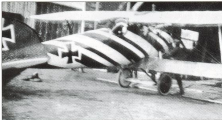
This Albatros D V was flown by Fritz Rumeys in Jasta 5 . While not a brilliant photo, it does show the black and white candy stripes to good effect. Note too that even the struts and wheel covers were painted alternatively black and white – all designed to throw off the aim of a pursuing pilot by optical illusion. The two white stripes on the green horizontal tailplane were unique to Rumeys's machine (G VanWyngarden collection)
