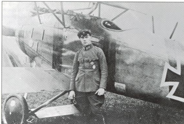
Kurt Wüsthoff flew this black spiral-marked Albatros D III (OAW) with Jasta 4 in 1917. It features dark grey or even black wheel covers, and otherwise standard camouflage. The black spiral band around the fuselage was the unit marking of Jasta 4 (G VanWyngarden collection)
