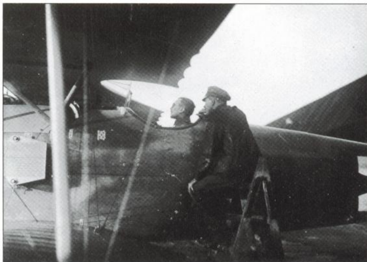
Rudolf Berthold is seen in the cockpit of his Albatros D II D.1717/16 at Bühl airfield whilst serving with Jasta 14 . The aircraft has bears no specific markings other than the ply fuselage was probably stained a reddish brown colour. Note the fuselage radiators which caused drag and were mounted on the wing in later models of the Albatros ( G VanWyngarden collection )
