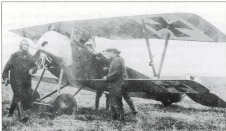
This Nieuport 11 (N1324) of Escadrille N35 was shot down by Kurt Student on 6 July 1916. Quickly repaired, the fighter was later flown by the German pilot in combat. Note that a Spandau machine-gun, larger windscreen and an anemometer ASI (on the left 'V'-strut) have been fitted by the Germans (via Greg VanWyngarden)
