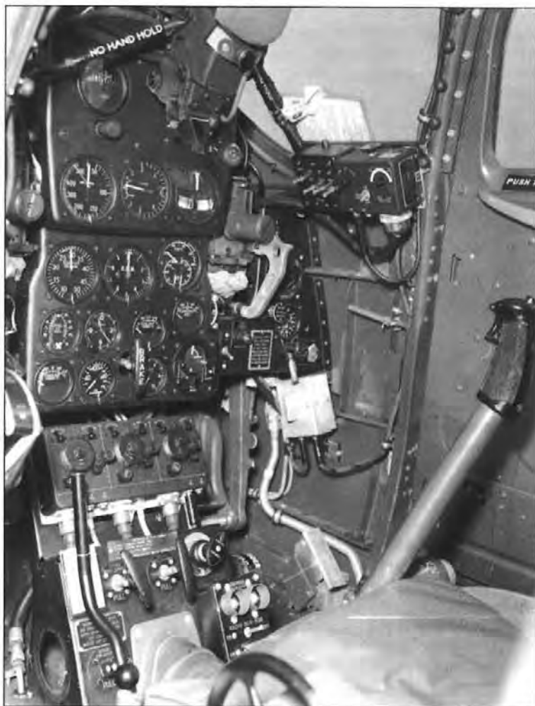
The cockpit of a standard P-39D. The Airacobra's cockpit was designed specifically for a 5 ft 8 in pilot who weighed 200 lb when equipped with his parachute and full flying gear. For larger pilots the cockpit was definitely on the cramped side, but the wind-down windows in the entry doors helped a little bit when the aircraft was on the ground. This unique window layout was one thing about the P-39 which really stuck in the memory of most pilots that flew it. 'Bud' Anderson remembers, 'You could taxi the thing while resting your elbows on the sill, like cruising the boulevard on a Saturday night' (via Michael O'Leary)
