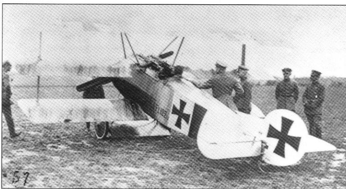
On 31 August 1917, Anthony Fokker demonstrated his new F I 102/17 to a collection of dignitaries at Jasta 11's airfield at Marckebeeke. Here, Fokker is seen in the cockpit as Maj-Gen von Lossberg rests his arm on the fuselage next to Manfred von Richthofen, leader of JG I. Next is Karl Bodenschatz, JG I's adjutant, and Ltn Hans Adam of Jasta 6. This view clearly shows the curved leading edge of the tailplane, which was one of the distinguishing characteristics of the pre-production F I machines. These F Is were probably finished in an overall coat of undersurface light blue – over this the Fokker camouflage of a greyish olive-brown was applied, resulting in a typical streaky finish to the uppersurfaces (via Van Wyngarden)
