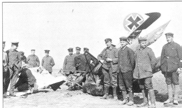
By the time this photograph was taken the wreckage of Lothar's top wing has been removed, revealing the red cowling and cabane struts (via VanWyngarden)
