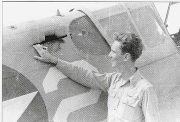
1Lt John J Stefanik of the 66th FS/57th FG examines combat damage that he picked up in P-40F 'White 72' during a scrap with Bf 109s. The tough Warhawk lost its radio, but it brought Stefanik home unhurt (via Dan and Melinda Shobe)
