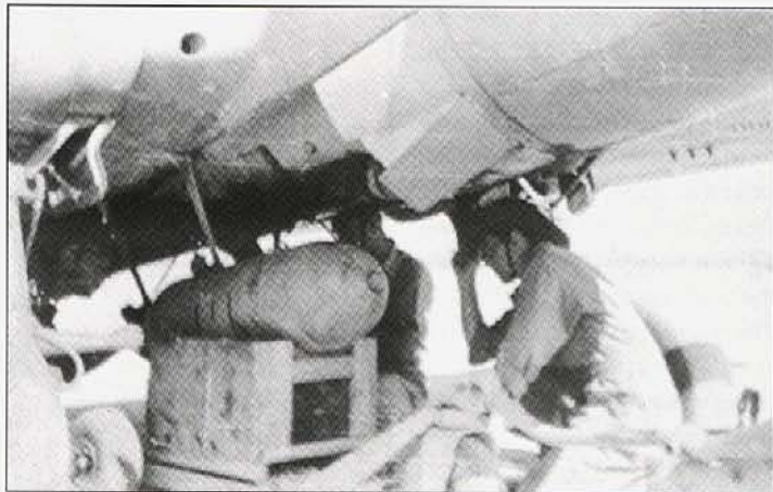
Armourers from the 66th FS/57th FG use a home-made lifting rack to ease the mounting of a 500-lb bomb under the belly of a P-40K Warhawk. The three small protrusions under the wing at right are attachment points for smaller 40-lb weapons (Lou Lederman)
