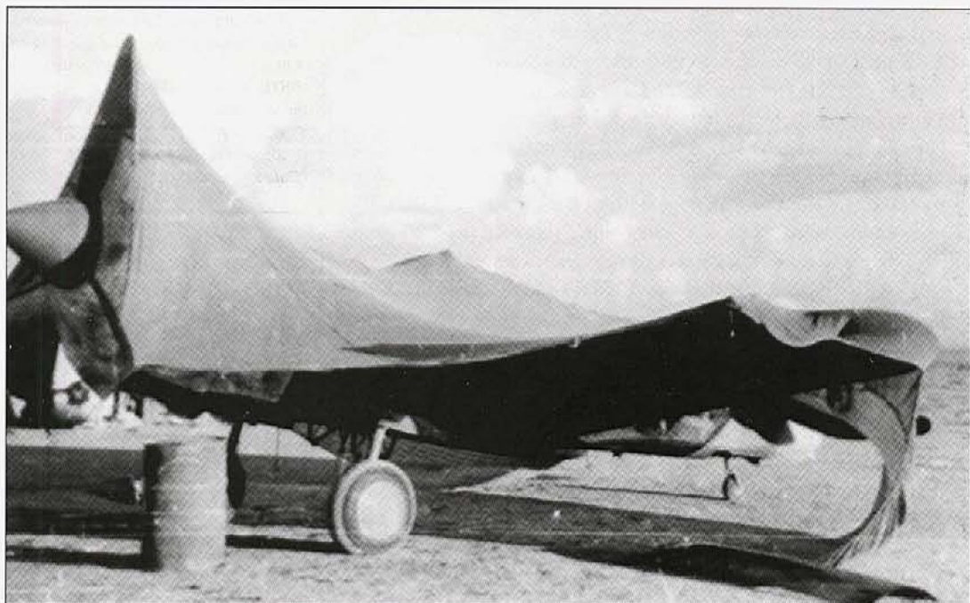
Blowing sand and dust played havoc with the working parts of aircraft in the desert. This 66th FS/57th FG Warhawk wears a canvas 'cocoon' for protection (Lou Lederman)
