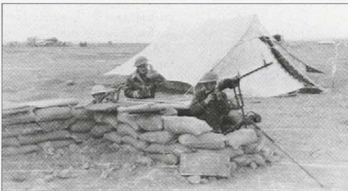
S/Sgt Lou Lederman, a crew chief in the 66th FS/57th FG, mans the anti-aircraft gun he rigged by mounting a German Spandau machine gun from a downed Stuka on an upturned bicycle fork, attached to a tripod! ( Lou Lederman )
