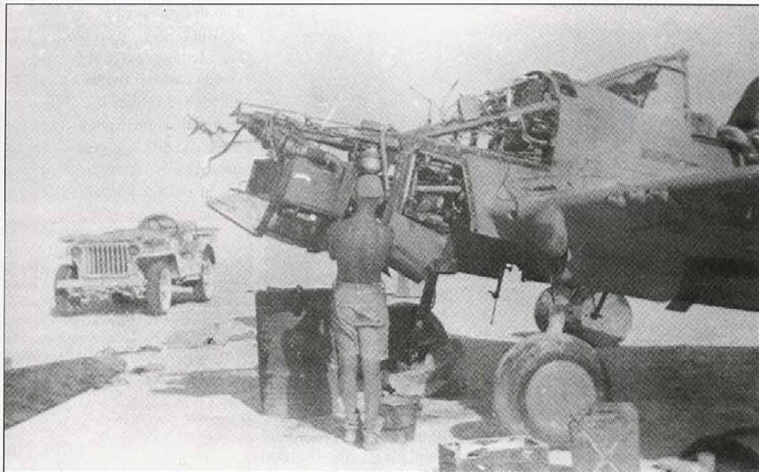
Groundcrews toiled under brutal conditions in North Africa. Here, a bronzed mechanic dressed only in shorts, shoes and a cap works on a P-40F that is undergoing an open-air engine change ( Dale Deniston )
