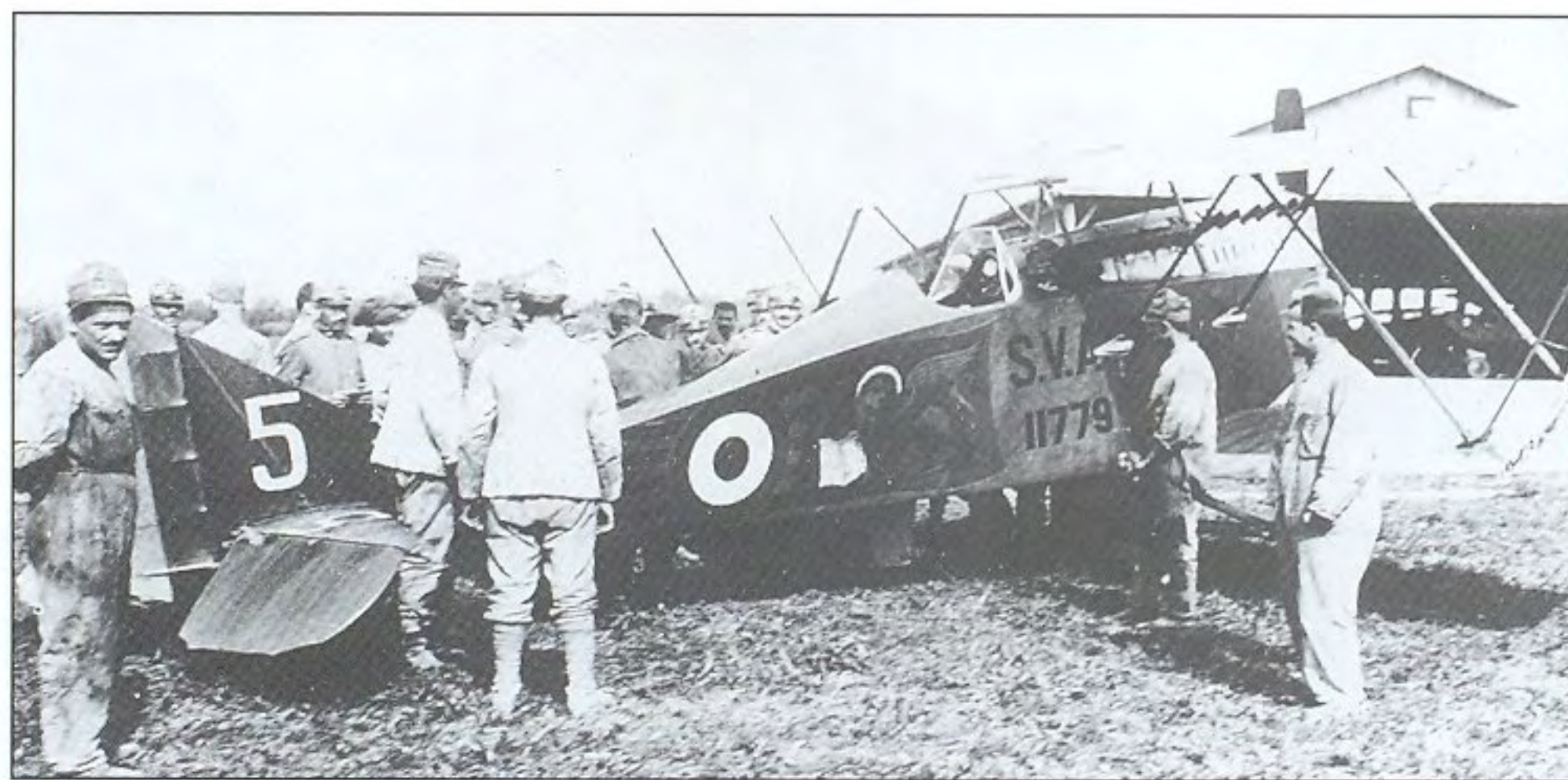
The Ansaldo SVA-5 lacked the agility for effective use as a pure fighter, but possessed the speed and range to operate usefully in the escort fighter and high-speed reconnaissance roles. As indicated by the 'Lion of St Mark' insignia on the sides of the fuselage (which was of inverted triangular section to the rear of the cockpit), this was a machine of the 87 a Squadriglia 'La Serenissima' associated with Venice (Bruce Robertson)
