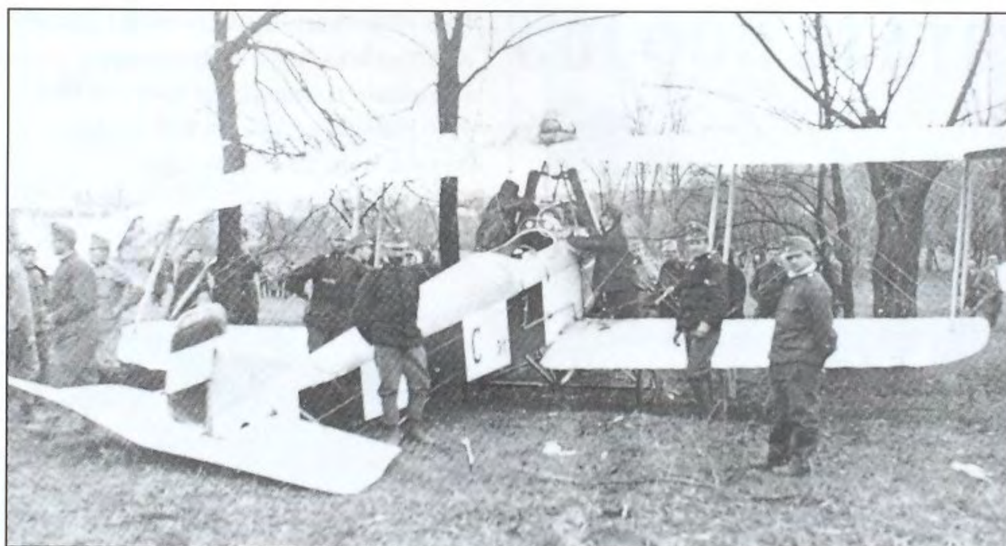
Seen with minor damage after running into a tree on landing, this Lohner Type C (C.51) two-seater was on the strength of Flik 15 on the Eastern Front in 1915. The aeroplane carries the red/white/red stripe marking introduced in 1913, and later became a B II (U) with the revised serial 12.51
