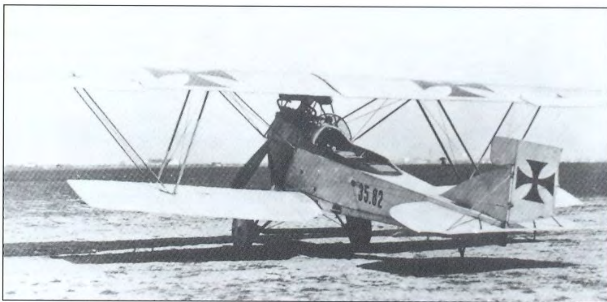
In common with a number of other aircraft designed and built in Austria-Hungary, the Knoller B I two-seater had a high forward decking over its inline engine, in this instance a Thöne & Fiala-built training machine in the 35.8-series with a 74.6 kW (100 hp) engine. In combination with the large windscreen, this provided the crew with good protection from the slipstream (Bruce Robertson)
