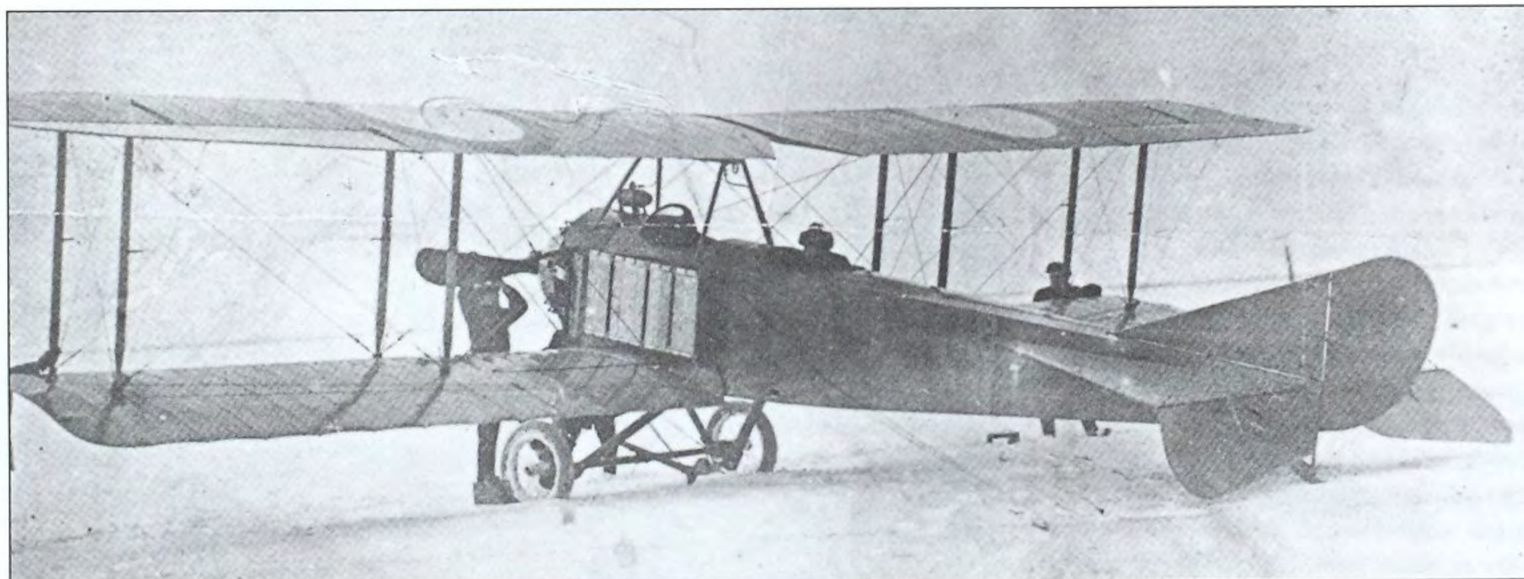
The Lebed' XII was an improved version of the Lebed' XI in the two-seat reconnaissance and artillery observation role with a wing cellule of smaller area to enhance agility and performance and at the same time to reduce the type's tendency to 'float' on landing (Bruce Robertson)
