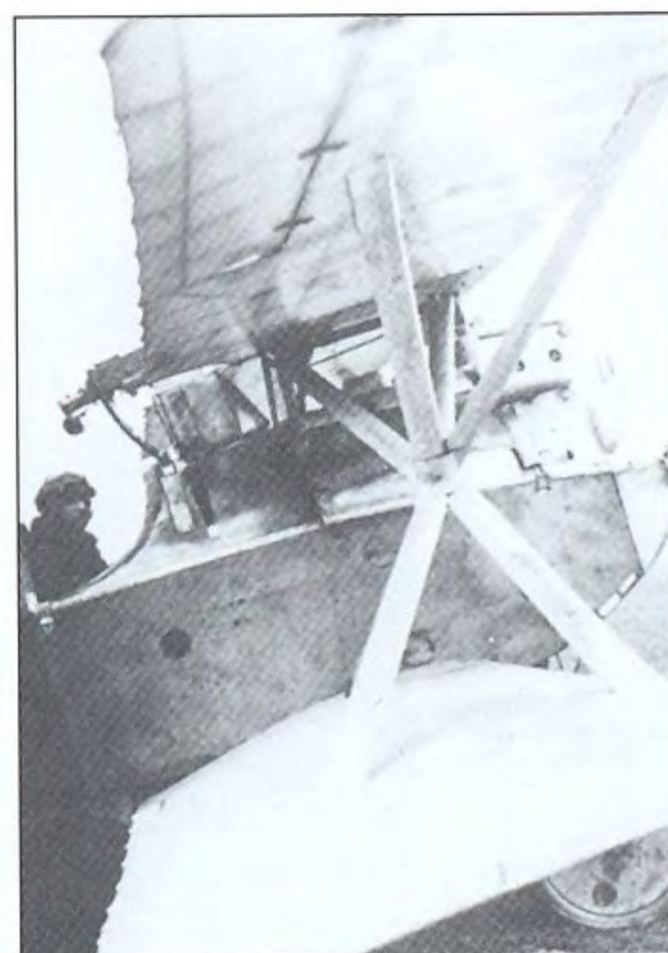
Raoul Stojasavljevic in his Hansa-Brandenburg D I 'star-strutter' fighter (28.30) of Flik 16 on Villach airfield on 14 August 1917. This far-sighted pilot was a pioneer of high-speed photo-reconnaissance (using a captured Italian camera in a fuselage compartment of his aeroplane), and personalised features of this machine include the large windscreen, and the curved rail allowing him to bring down the rear of the two fixed forward-firing machine guns so that he could clear jams
