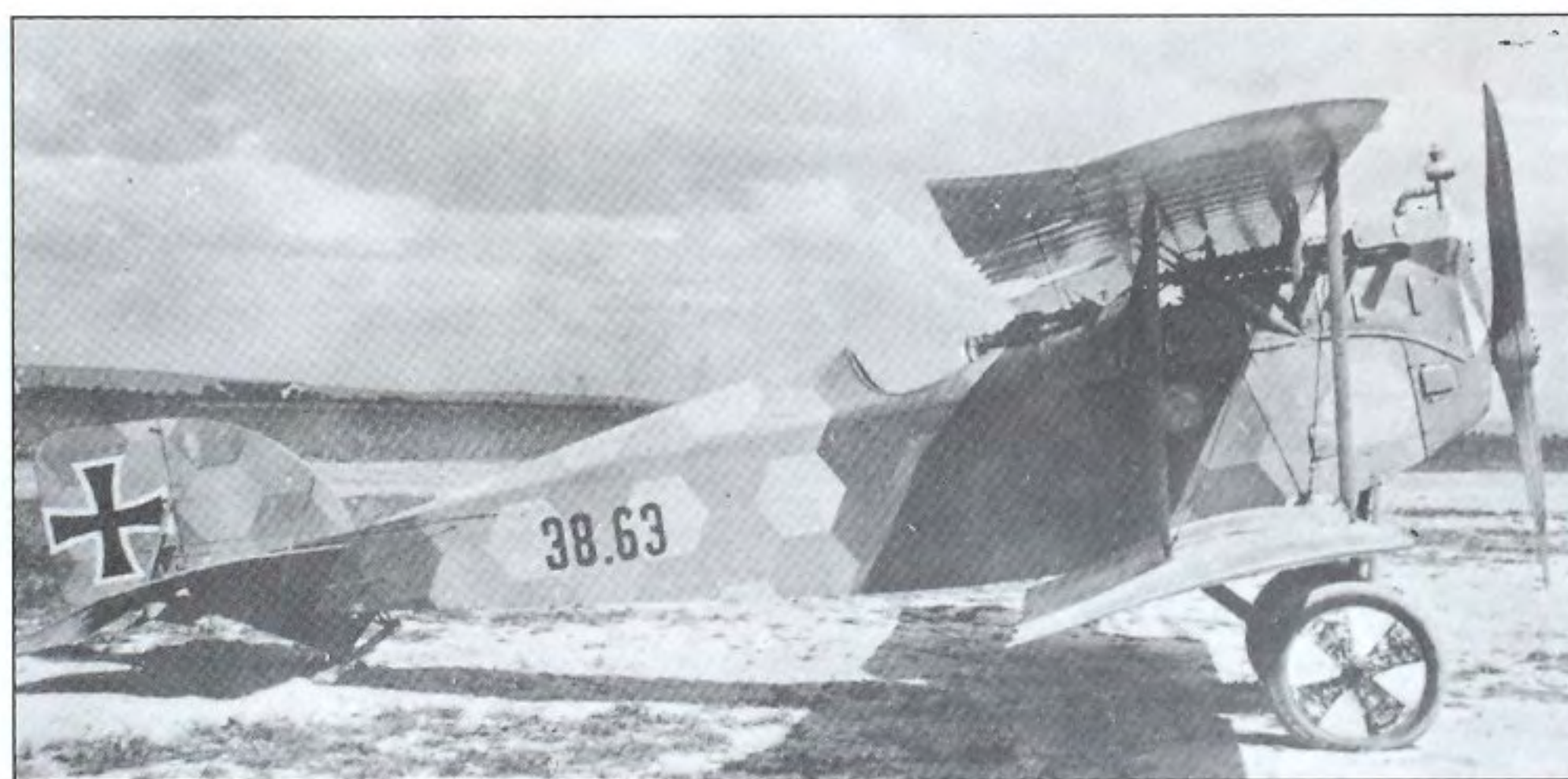
One of the mainstays of the Austro-Hungarian army air service's fighter arm was the Aviatik D I. This photograph shows 38.63 of the 38-series, powered by a 138 kW (185 hp) Austro-Daimler engine. 38.63 crashed as result of wing failure on 15 July 1918 injuring the pilot, Korporal Mazarlet of Flik 74 (Bruce Robertson)
