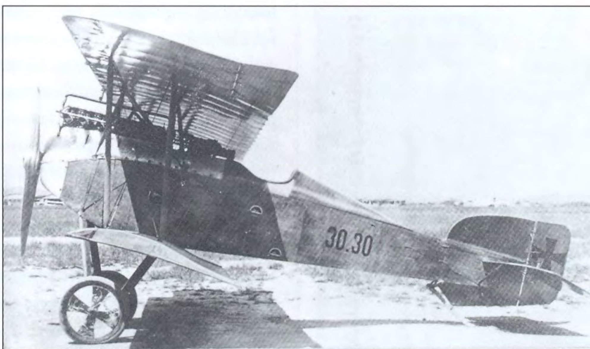
The serial 30.30 identifies this single-seat fighter biplane as the Aviatik D III, a type developed with a 171.5 kW (230 hp) Hiero inline engine and evaluated at the Aspern fighter competition of July 1918 as a candidate to replace obsolescent types such as the Aviatik D I (Bruce Robertson)
