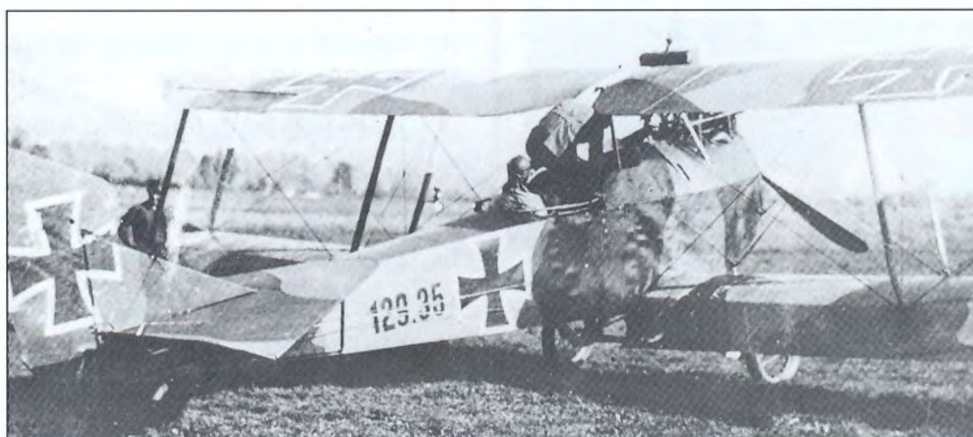
This Phönix-built Hansa-Brandenburg C I (129.35) was powered by a 149 kW (200 hp) Hiero inline engine and sported non-standard camouflage. The aeroplane was released to Flep 1 in April 1917 before being passed to FIG 1 (later Flik 101G ) and then, during 1918, to Flik 21D and finally Flik 23D (Bruce Robertson)
