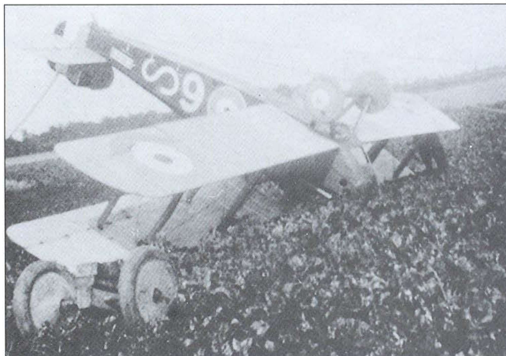
American pilot Lt D C Mangan, turned '6' (C8109) over in no-man's land on 25 August when he was forced to crash-land it. He had scored two victories in this machine up to this point in the fighter's short career. Note the wires attached to the tail in order to pull the machine back onto its undercarriage, and the 'dolly' in the foreground to wheel it back to the nearby airfield
