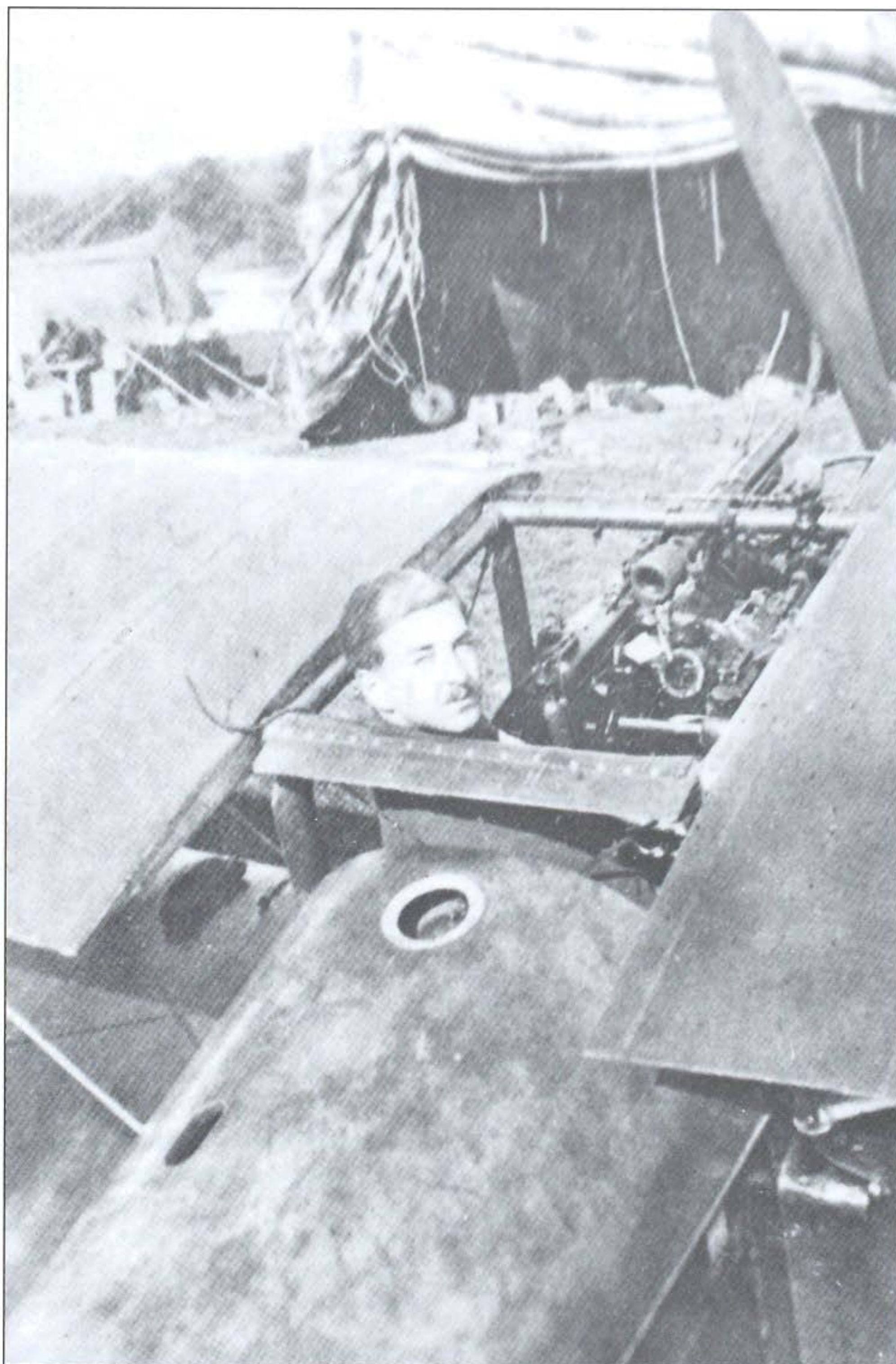
No 87 Sqn five-kill Dolphin ace Lt C E Worthington relaxes in the cockpit of his fighter in France in 1918. This view clearly shows just how good the vision was for a Dolphin pilot. Note the Aldis gun sight, and the 'C Flight' wheel (painted all white) propped up inside the makeshift canvas hangar. Immediately behind the cockpit is the filler cap for the fighter's seven-gallon gravity tank
