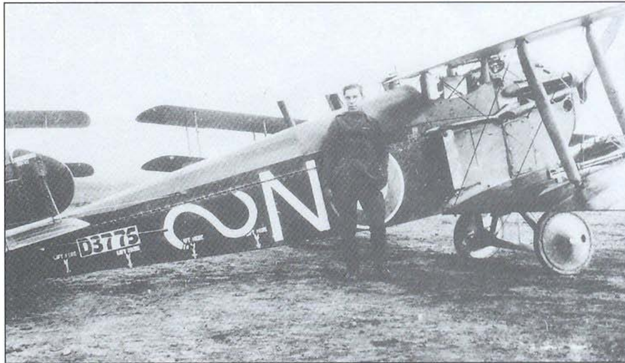
No 87 Sqn's Lt A J Golding and his D3775. Note that he has added an 'eye' and a 'rattle' to the squadron marking, turning the 'lazy S' into a snake. Post-war, the snake insignia became the basis of the unit's crest. A small repeat serial number can just be made out under a white tape on the tail-fin. This machine also features extra Lewis guns on the lower wings, with the cord for firing these weapons going into a small hole by the wingroot
