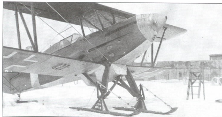
A cannon-armed Bk 534 fitted with Slovak-made skis has its engine run-up at Trencianske Biskupice aerodrome. Skis were used in field conditions only during 1942, when No 11 Sqn fought Soviet partisans in the Ukraine and Byelorussia
