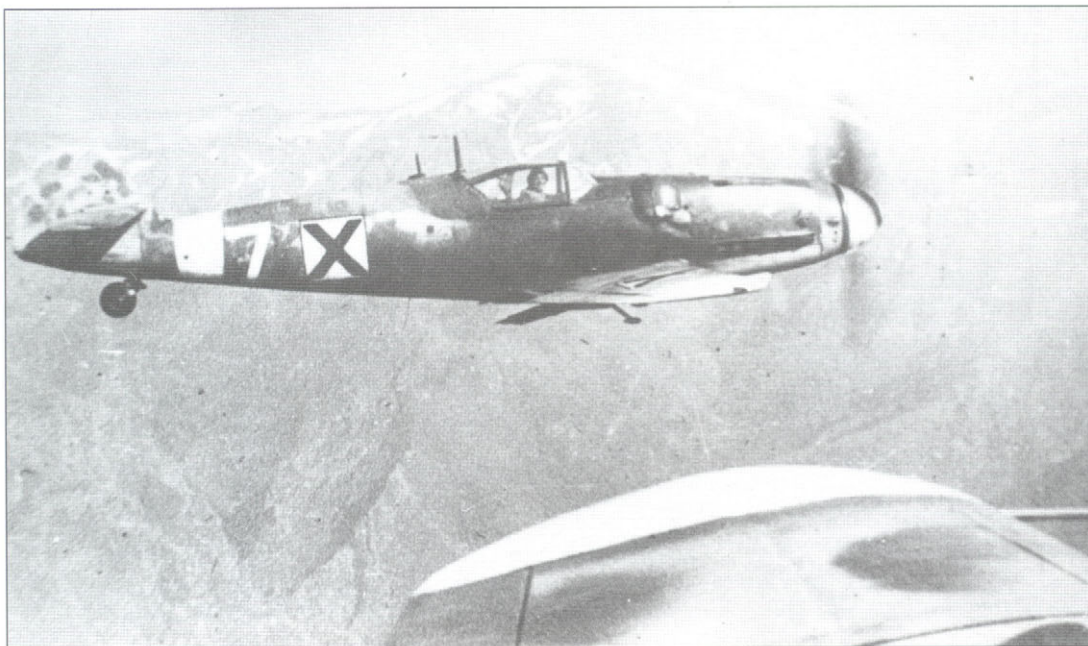
Bf 109G-6/trop 'White 7', with its distinctive Erla hood, was part of the last batch of Messerschmitt fighters delivered to Bulgaria in the summer of 1944. It is seen here on patrol with poruchik Somov of 3.6 Orlyak at the controls
