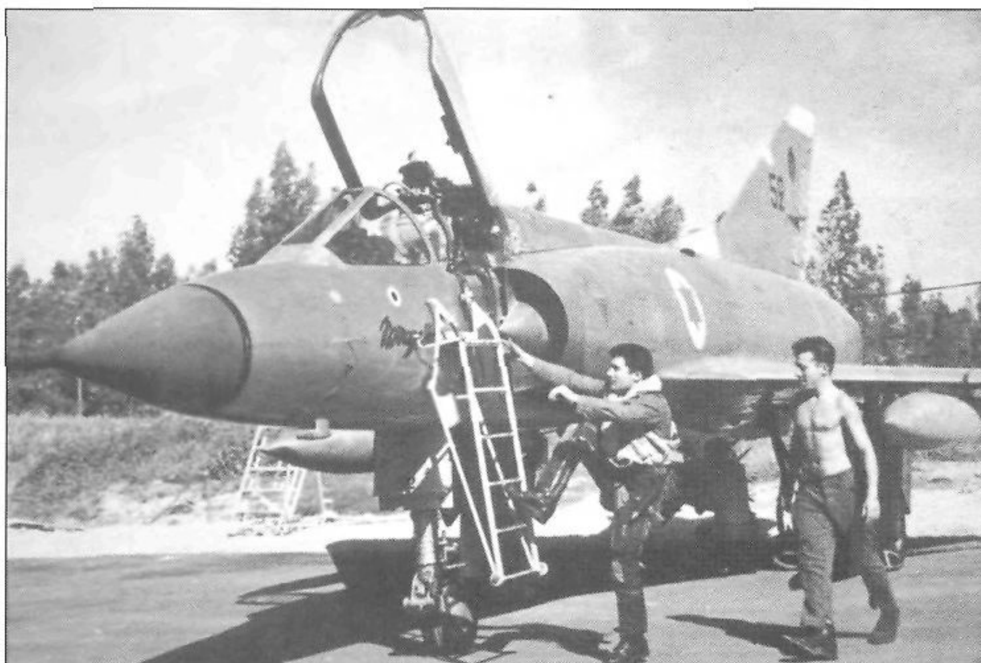
Scramble! No 101 Sqn pilot Avshalom Ran dashes to Shahak 52, which is armed with an R.530 Yahalom AAM on the centreline pylon. The jet also carries a ubiquitous 500-litre supersonic fuel tank under each wing
