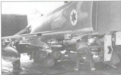
No 107 Sqn groundcrew prepare Kurnass 122 for a mission during the Yom Kippur War. Note the absence of detonators in the cluster-bomb units, which were only installed at the last moment. The housing for the battle damage assessment camera can be seen below the wing root
