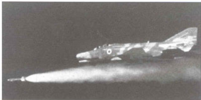
Kurnass 101 test-launches a red-painted Rafael Python 3 AAM. The Python 3 entered service with No 69 Sqn in 1978, succeeding the AIM-9D as the preferred close-range air-to-air missile. The F-15's service introduction two years earlier had resulted in the AIM-7's progressive removal from the list of Kurnass weapon options
