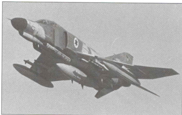
No 201 Squadron Kurnass 673 (ex-68-0525) takes off during the Yom Kippur War in air-to-air combat configuration, carrying four AIM-9Ds, two AIM-7s, an electronic warfare pod and three external fuel tanks. This aircraft was lost in air combat on 11 October 1973
