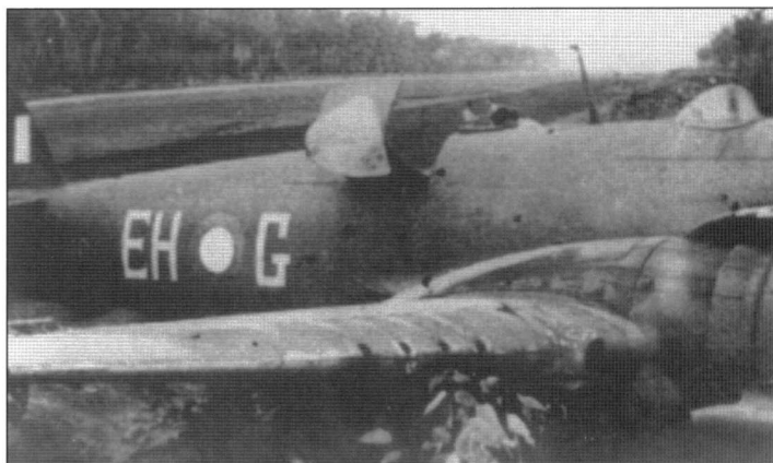
During his 9 October 1943 combats, 'Butch' Gordon's Beaufighter was hit, causing damage to an engine, hydraulics and control surfaces. After a two-hour flight back to Australia, he had to crash-land at Livingstone airstrip. Having sustained over 100 cannon shell and bullet holes, A19-40/EH-G was fit only for scrap (R Jordan via P H T Green)
