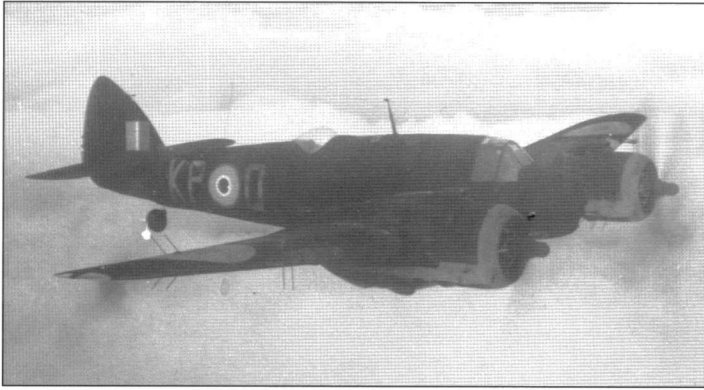
This splendid view of No 409 Sqn's Beaufighter VIF KP-Q was taken around September 1942, and shows all the various transmitting and receiving radar aerials to advantage (D M Dixon)
