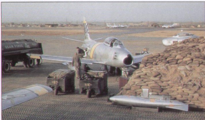
A 39th FS Sabre is readied for its next mission out on the Suwon flightline. The jet is being filled with JP-4 from the refuelling truck parked to the left of the photograph. The high-walled sandbag revetments are clearly visible in this shot (Ron Wilson)
