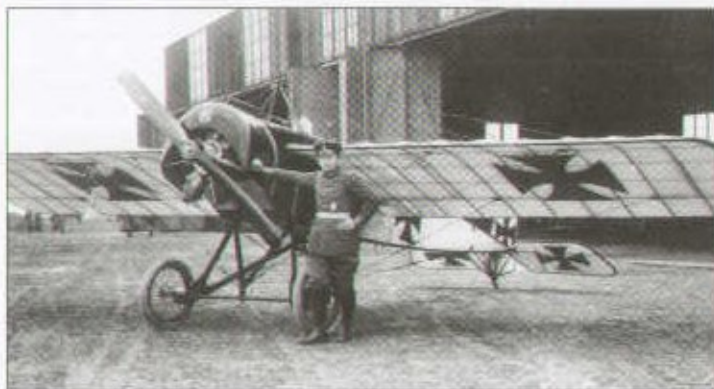
Taken on the same occasion as the photograph above, this view of Kissenberth with his Pfalz E I at KEK Ensisheim reveals the circular Pfalz nameplate on the front of the cowling (an imitation of Morane-Saulnier practice). The E I was the first Pfalz product armed with a synchronised machine gun. The translucency of the bleached white fabric is evident. The multitude of national markings was perhaps deemed necessary to prevent confusion with French Morane-Saulnier machines
