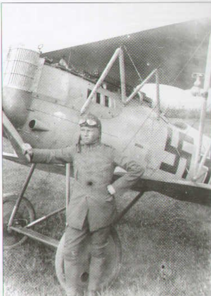
An unidentified pilot of Jasta 77b strikes a confident pose with a Pfalz D XII thought to be 394/18. This was an early-production machine with the initial style of fin and rudder, and it also boasted the Staffel markings of a blue nose and tail. The black(?) swastika was a personal insignia, and at this time was known only as a common good luck totem, with no political significance. An anemometer has been affixed, and a rectangular foresight is also in place (SHAA B89-4338)
