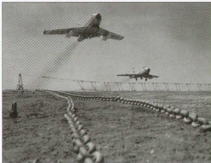
When a Sabre returned from a mission to Kimpo AB with its hydraulics shot out, the emergency safety barrier seen here would be raised at the end of the runway to prevent the pilot and his jet from running off into the sand and dirt. The two F-86s shown here, both fitted with full external tanks, are destined for 'MiG Alley' (Bill Graski)
