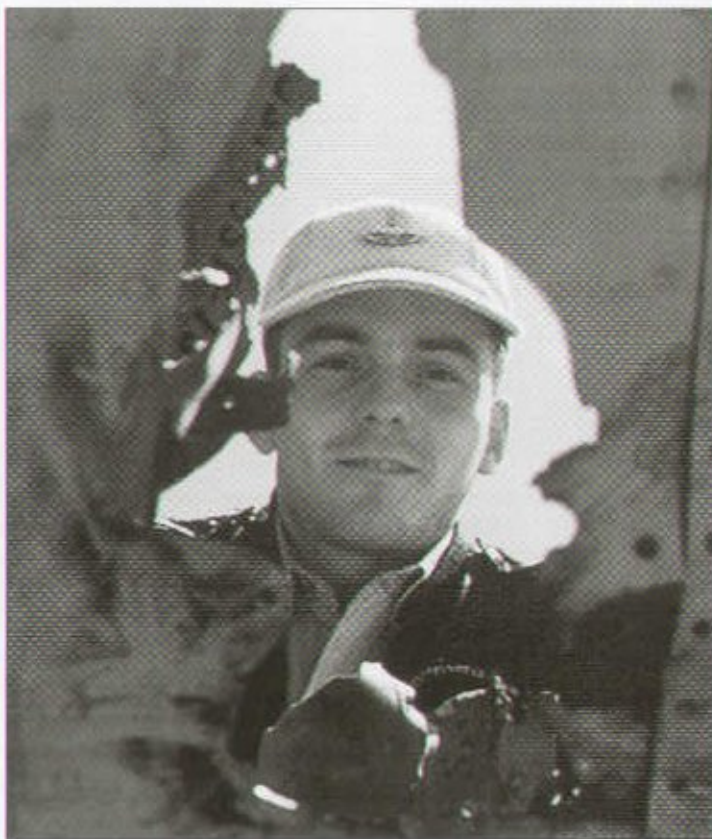
335th FS pilot 1Lt Martin Bambrick peers through a large hole in the wing of his Sabre made by a 37 mm cannon round fired from a MiG-15 in June 1952 (Martin Bambrick)
